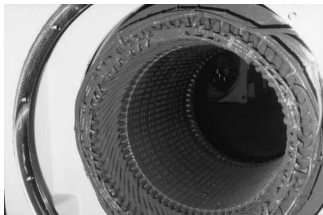
Figure 3. Photograph of a complete form-wound stator.
