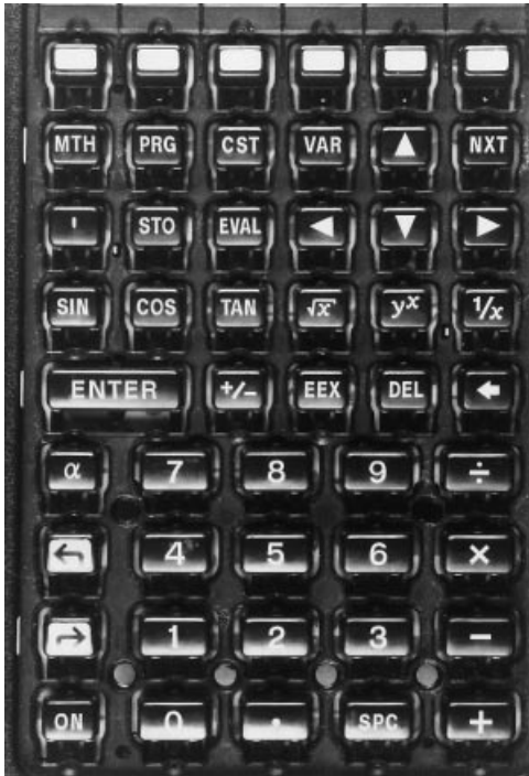
Figure 5. Hinged plastic keys provide tactile feedback to the user.
