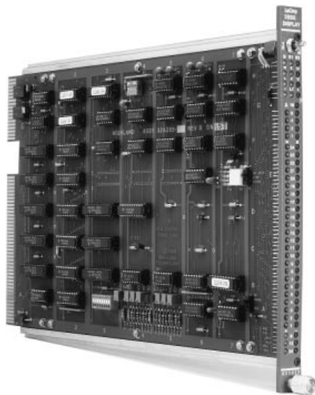
Figure 1. A typical single-width CAMAC module. The 86-contact dataway connector is on the left. Above the dataway connector there is another edge connector in the free access area at the rear of the CAMAC crate. This area is available for any user-defined purpose. (Courtesy of LeCroy Corporation and Highland Technology.)
