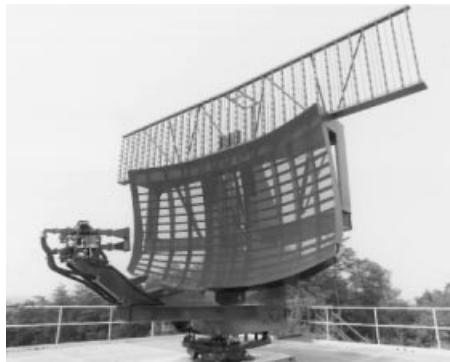
Fig. 13. The Northrop Grumman ASR-12 is a modular, fully solid-state, S-band airport surveillance radar. It uses a moving target detection scheme that combines adaptive Doppler filter and fine-scale clutter mapping to enhance the returns from tangential targets. Photo courtesy of Northrop Grumman Corporation.
