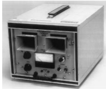
Fig. 24. A K_u -band electronic moving target simulator. One horn receives the transmitted signal, which is mixed down with one STALO and mixed back up with another matched STALO. A discriminator circuit provides a visual indication of target Doppler frequency and direction. An attenuator provides control over the radar cross section of the return signal.
