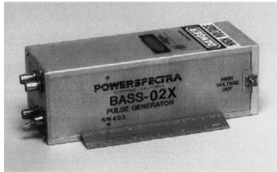
Fig. 19. The PowerSpectra BASS-02X is a bulk avalanche semiconductor switch activated by a semiconductor laser. Rise times are about 150 ps with a fall time of approximately 2 ns. Peak output power is approximately 2 MW, and average power is approximately 1.5 W. Prime power is 28 VDC, and the unit weighs approximately 2 kg. US Army photo.
