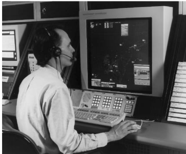
Fig. 32. A modern synthetic radar display that allows overlay of map data, weather data, air traffic controller to pilot data links, and IFF information to generate a powerful airspace management tool. Photo courtesy of Northrop Grumman Corporation.
