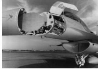
Fig. 12. The electrically driven antenna of an F-16 equipped with one of Northrop Grumman's APG-66/68(V) family of coherent radars. The radar supports 25 air-to-air, air-to-ground, and mapping modes that provide target detection, acquisition, and tracking in both benign and hostile electromagnetic emissions environments. Photo courtesy of Northrop Grumman Corporation.
