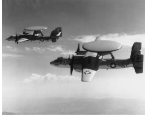
Fig. 26. A pair of Northrop Grumman E-2C Hawkeyes are easily identified by their distinctive 7.3 m (24 ft) diameter rotodomes, which contain both the low sidelobe radar antenna and the IFF antenna. A Lockheed Martin AN/APS-145 radar system automatically detects, identifies, and tracks targets at ranges exceeding 300 miles. US Naval Institute collection.
