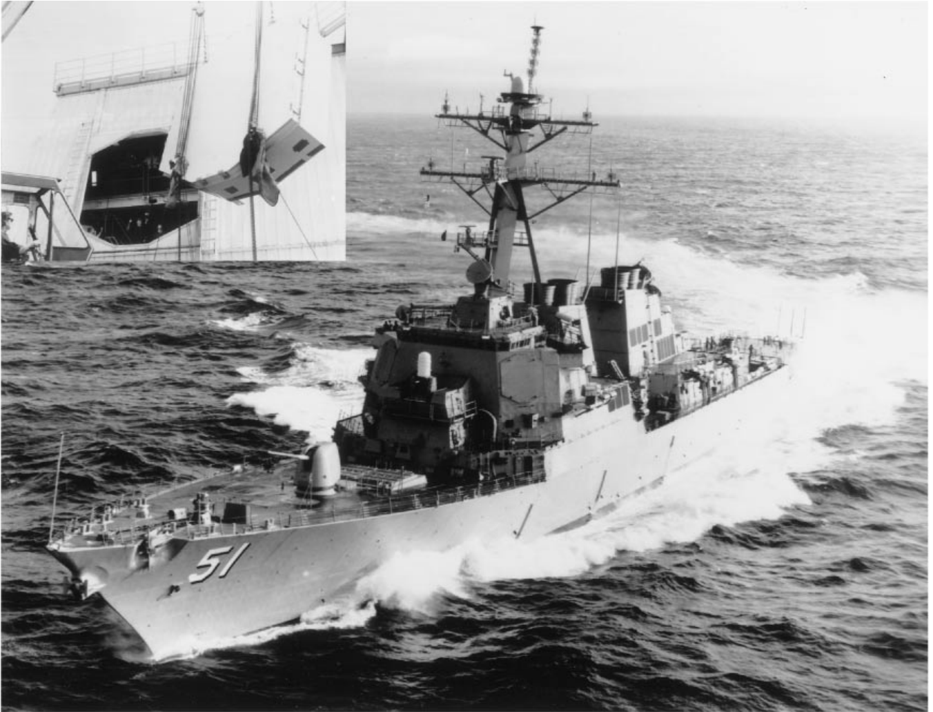
Fig. 28. The Arleigh Burke (DDG-51) Aegis system is based on the AN/SPY-1D multifunction phased-array S-band radar. The SPY-1 antennas are the octagonal panels on the corners of the deckhouse. The inset in the upper left shows an antenna being installed in a deckhouse. US Naval Institute collection.
