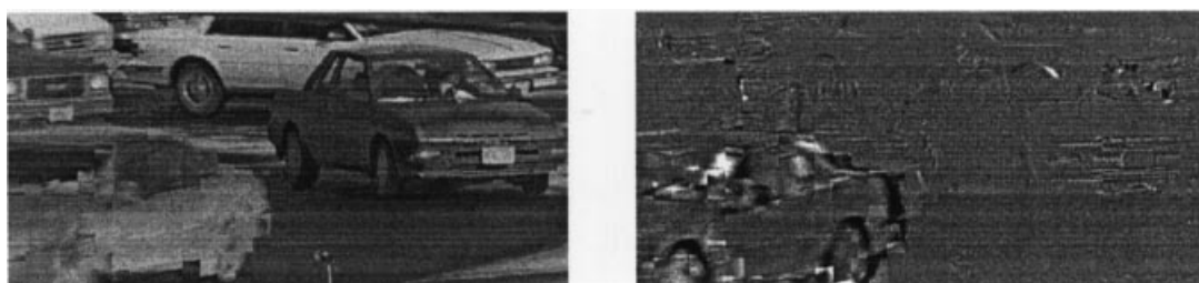
Figure 5. Block-based motion estimation and motion-compensation prediction applied to the two video frames shown in Fig. 1. The resulting prediction and error signals are shown on the left and right, respectively. The amplitude of the error signal has been scaled and offset so that gray corresponds to zero amplitude; white, a large positive amplitude; and black, a large negative amplitude.
