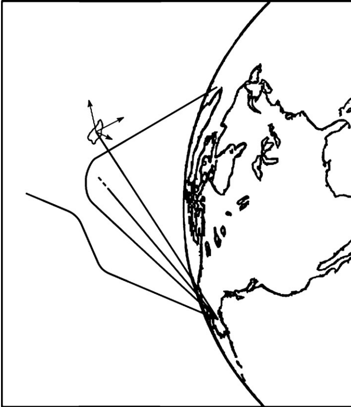
Figure 2. The four main mechanisms in MF and HF sky wave propagation: absorption, reflection, scatter, and penetration.
