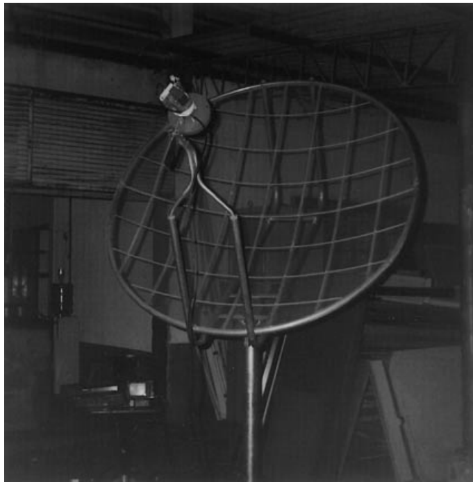
Figure 10. Just fully offset parabolic reflector antenna for satellite TV reception at C band, built and tested at the University of Brasilia. (Courtesy of Carlos Muller, University of Brasilia.)
