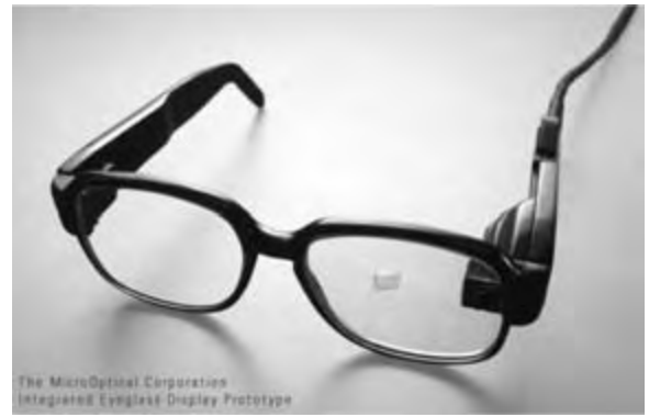
FIGURE 6.14 Prototype Integrated Eyeglass Display from MicroOptical Corporation. The mirror in the middle of one lens permits viewing of a video image produced in the structure on the left ear piece of the glasses. Image courtesy of MicroOptical.
