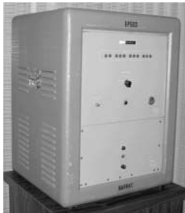
Figure 3.62: 1954 “DATRAC” 11-Bit, 50-kSPS SAR ADC Designed by Bernard M. Gordon at EPSCO
