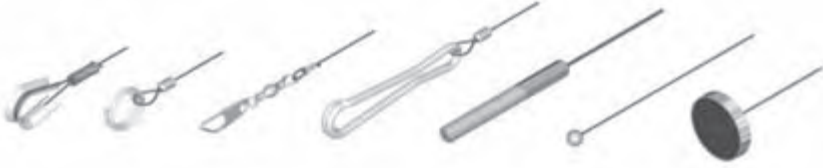
Figure 15.2.3: A few displacement cable terminations.
