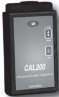
Figure 18.10.1: Sound level calibrator.
