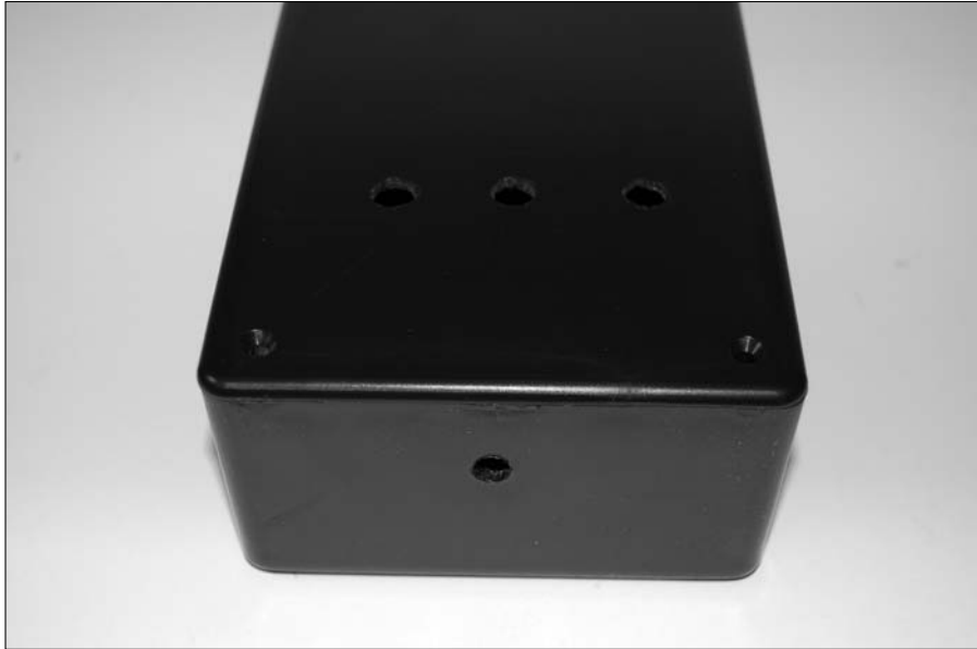
Figure 11-14: Drill holes for the LED and switches.
