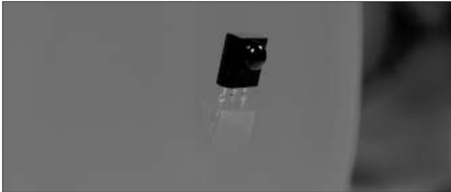
Figure 9-28: The IR detector mounted in the side of the pumpkin.
