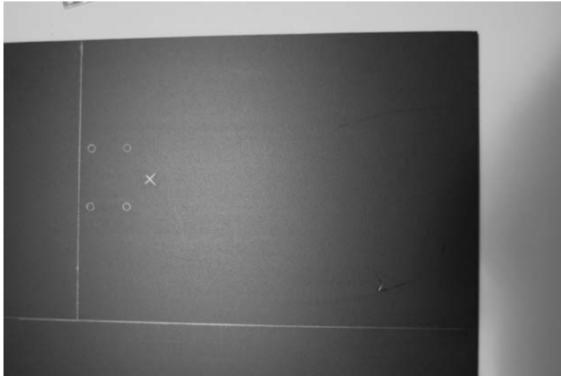
Figure 11-34: Mark the base for cutting and drilling.
