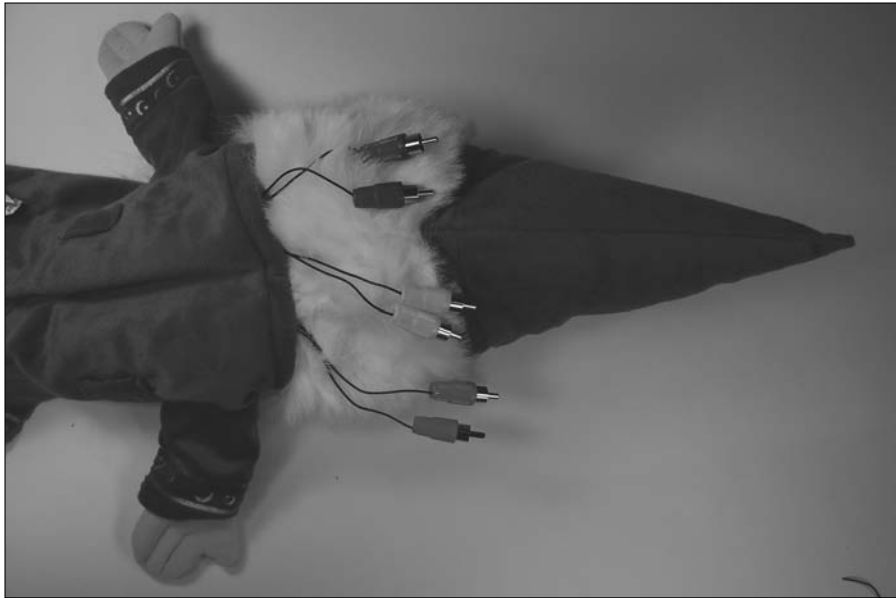
Figure 7-18: Place tactile switches in the puppet.
