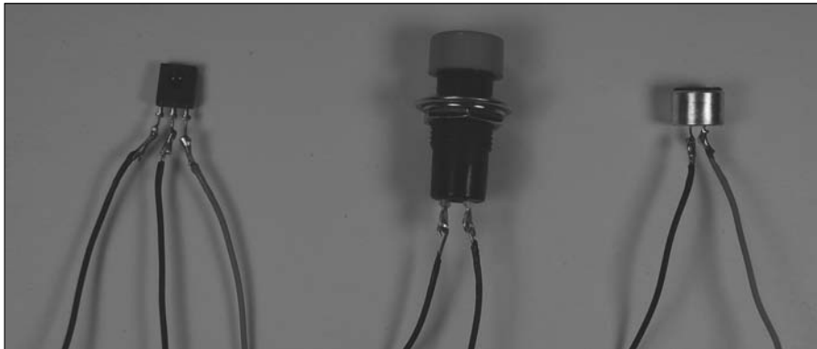
Figure 9-25: Wires soldered to the microphone, IR detector, and record switch.
