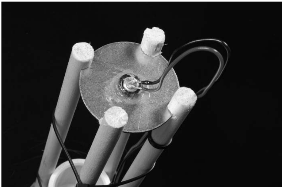
Figure 4-19: With the microphone cartridge in place.
