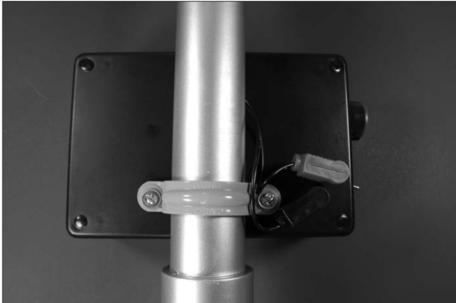
Figure 12-17: Box attached to the handle and phono plugs in place.
