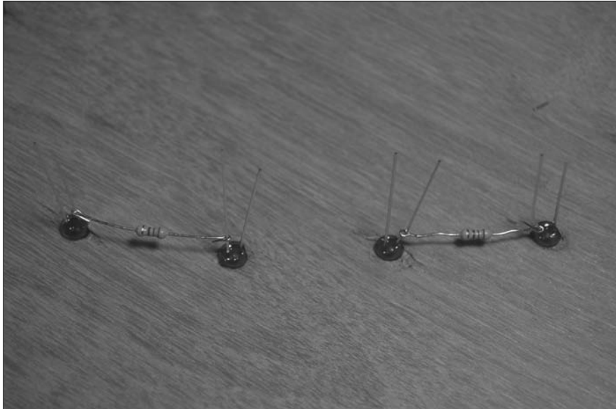
Figure 10-16: Attach resistors to LEDs.
