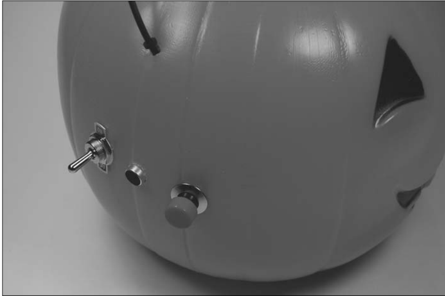
Figure 9-29: Switches and microphone mounted on pumpkin.
