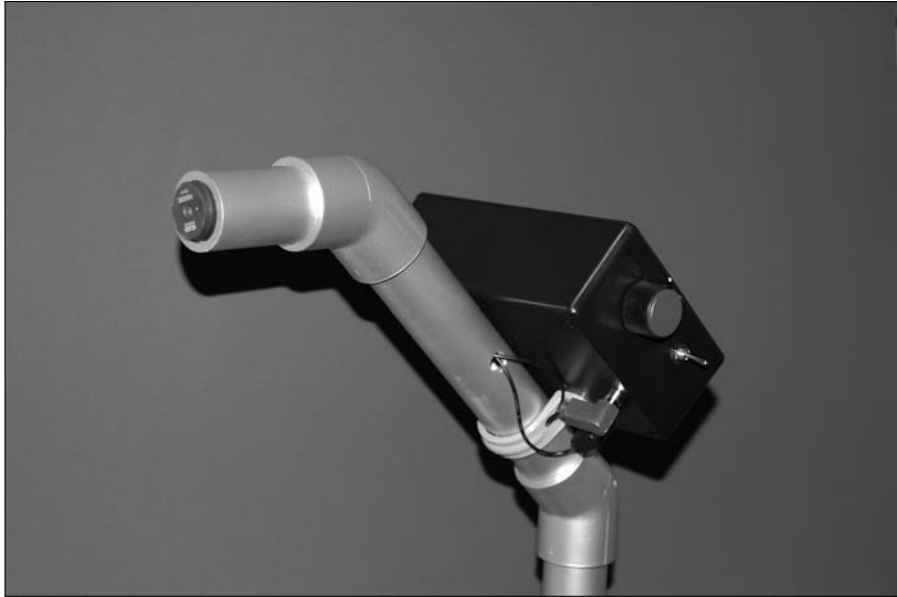
Figure 12-18: The finished metal detector.
