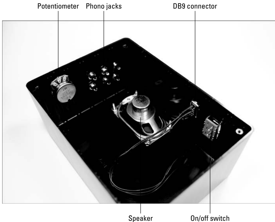
Figure 7-11: Mount components on the box.
