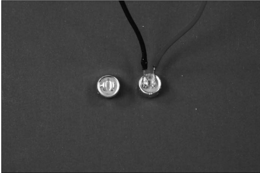
Figure 4-14: Soldering to flat contact pads.
