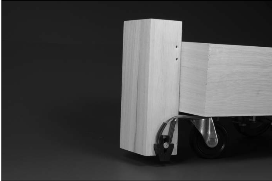
Figure 13-32: Keeping the sensors just off the floor allows Sam to spot the tape.
