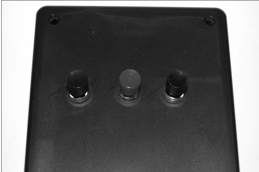
Figure 11-16: Transmitter box with switches installed.
