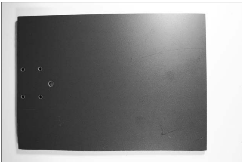
Figure 11-35: The base for the kart, all sawed, drilled, and sanded.
