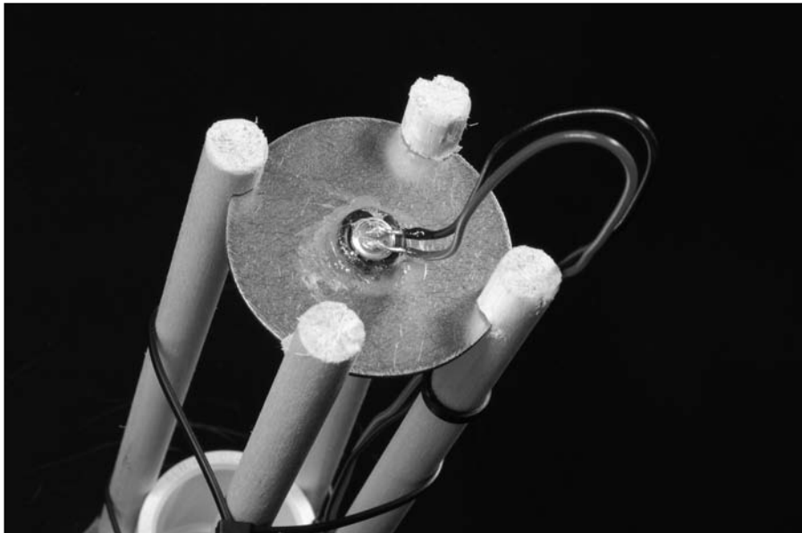
Figure 6-15: Microphone cartridge in place.
