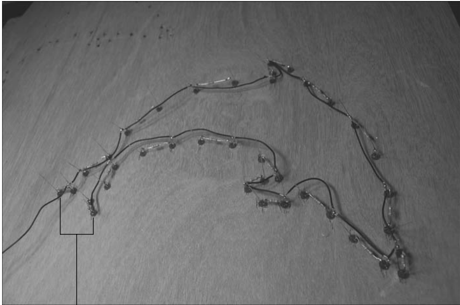
Figure 10-18: Black wires connecting short leads of LEDs.
