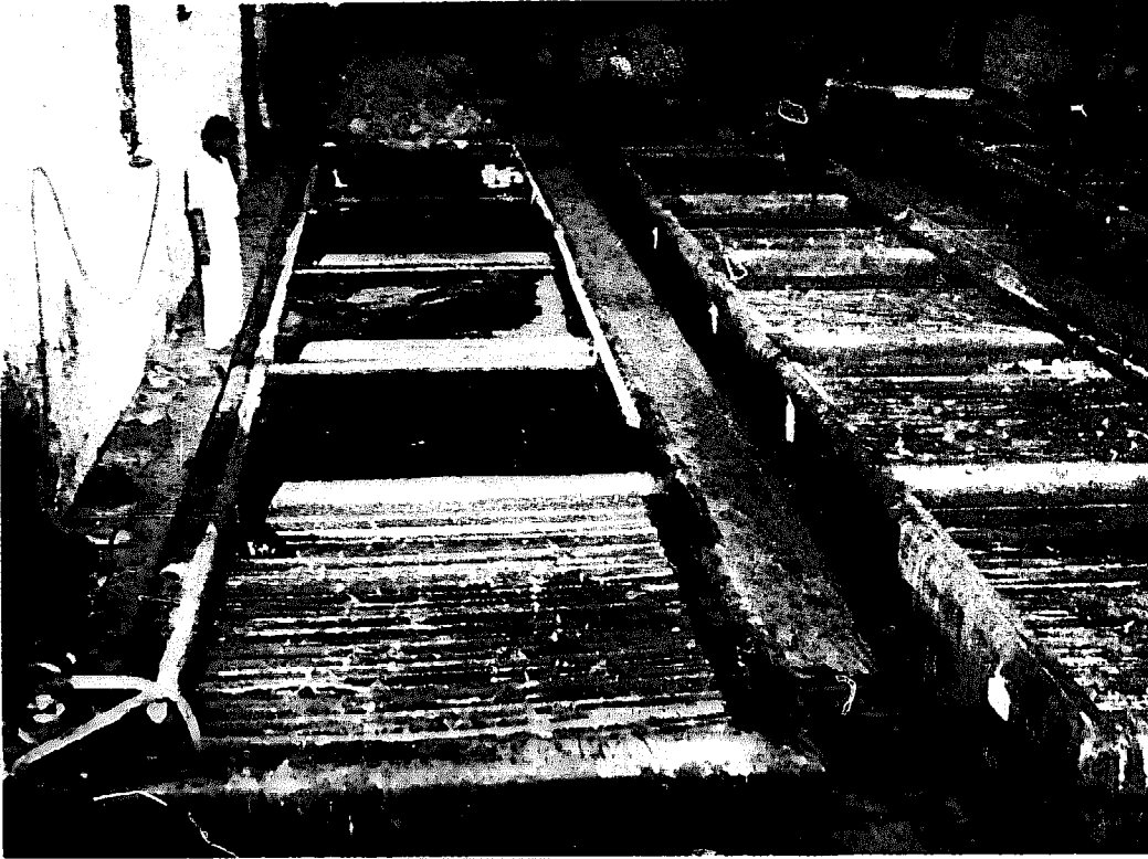
FIGURE 34. - Suspender vats as used in large tannery.
