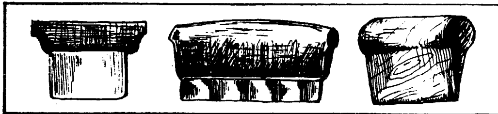
FIGURE 49. - Sketches of slickers which can be made of brass, steel, glass or hard wood.
