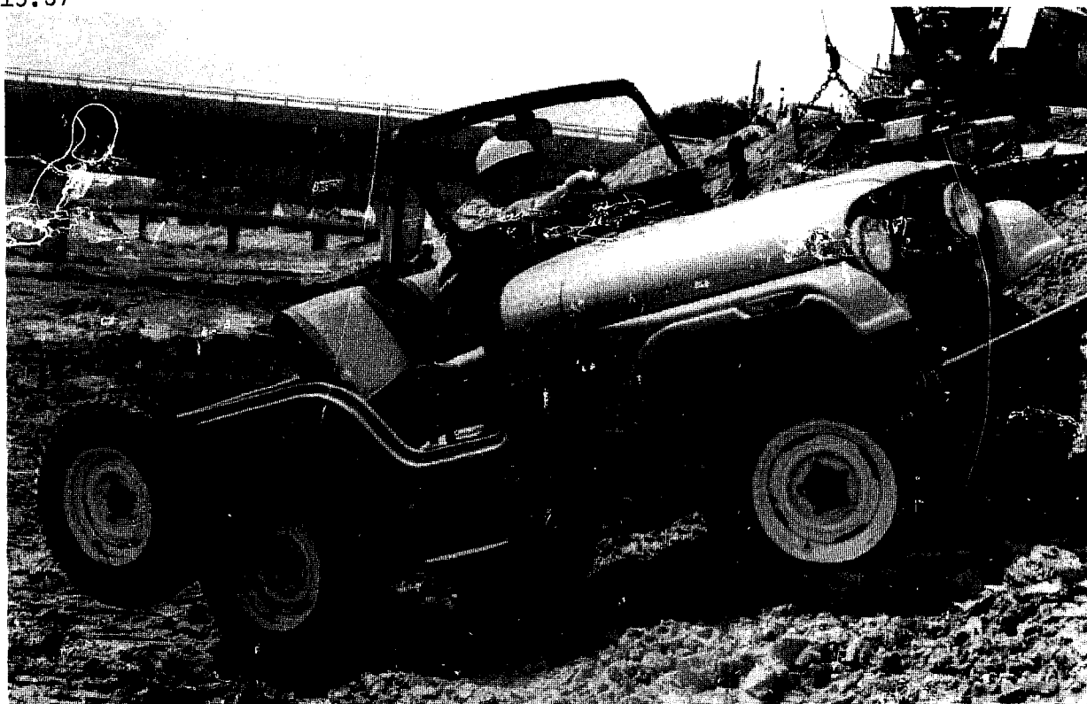
THE UNIVERSAL JEEP , based on the military vehicle of World War II, is one of the most widely accepted 4WD vehicles. Many manufacturers have produced the Jeep, but the basic design is little changed over the years. Although limited in size, it is capable of working in very difficult conditions. Parts are available all over the world. The same manufacturer also produces larger truck and carryall body styles.
