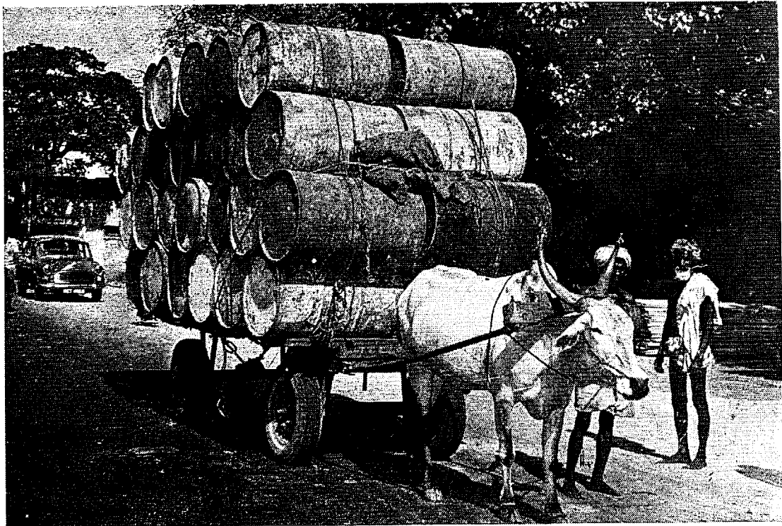
Four-wheeler carts—double bullock and single bullock drawn; one of the improvements brought about in some cities is the introduction of pneumatic tyred four-wheeler carts. As against the normal capacity of one ton of a traditional cart, such tyred carts carry as much as 4-5 tons on level roads. On a four-wheeler, that vertical load on the animal's neck and constant rubbing is eliminated.
