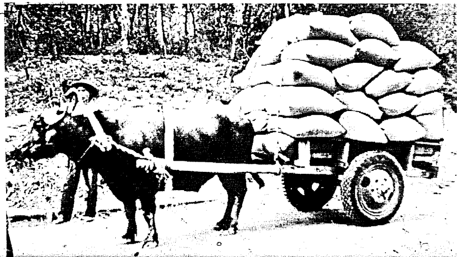
A single-harness buffalo-drawn cart in China. The cart is nominally improved with pneumatic tyres, and has a traditional yoke partially but simply modified for animal comfort. The single-harness cart is carrying about a tonne of bran or husk. Courtesy: W. Ross Cockrill; FAO; op. cit.
