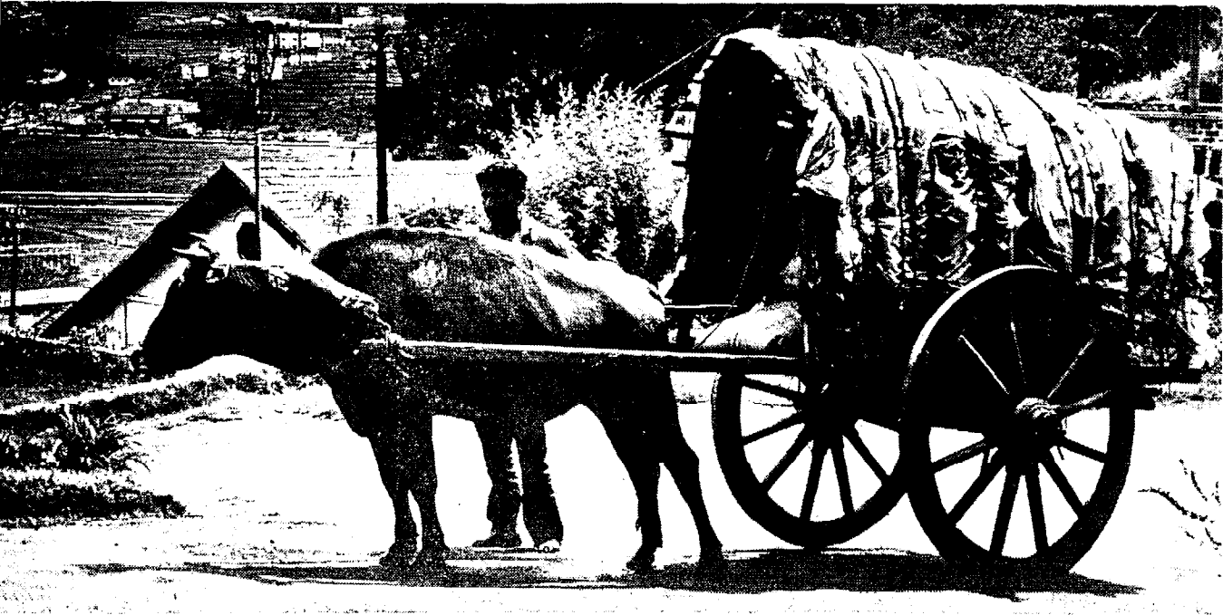
A plain buggy used in conjunction with discarded truck tyres and axle. Yoked to a buffalo, it is a common sight in the sugar-cane growing districts of U.P.
