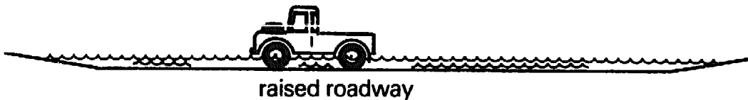
Figure 21(b). Wide crossing, shallow flood.
