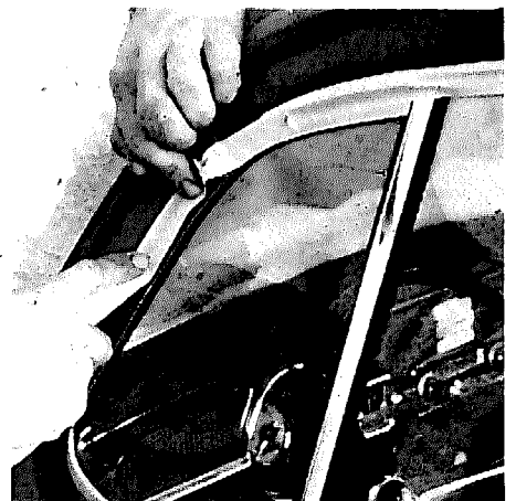
A taped-paper dispenser will make the masking job faster and easier.
