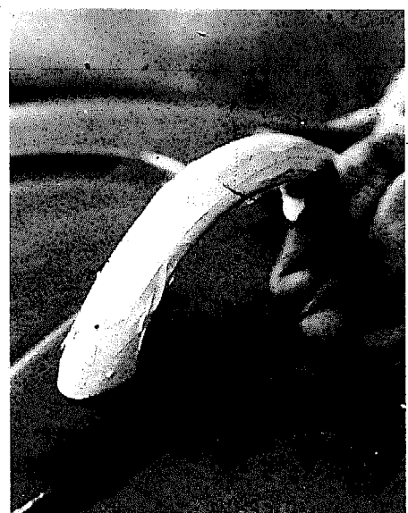
When masking trim, cover ends or complex curves, and then do the rest with as few pieces of tape as possible.
