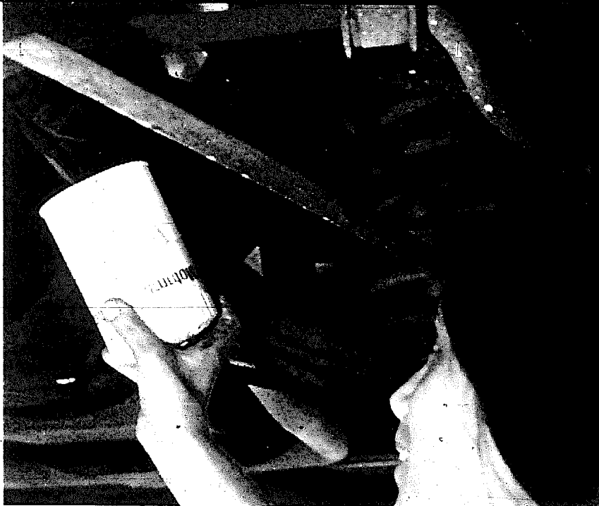
The new oil filter should be installed hand-tight only. If you put it on with a filter wrench, it'll take powers that you probably don't possess to get it off!
