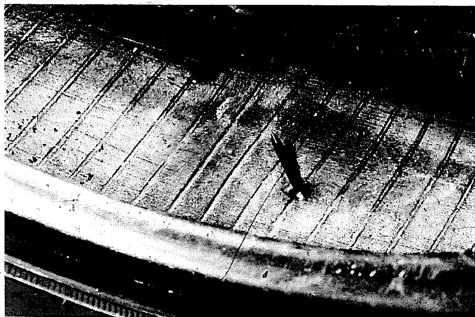
STEP 2: Locate and mark the damage. Remove the puncturing object and gently probe for evidence of separation and run-flat damage.
