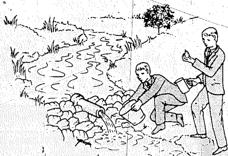
Fig 2.12. Measuring flow by damming and inserting a pipe
