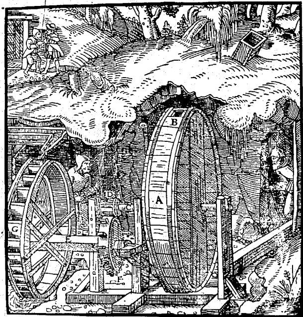
Fig 2.51 (a) Draining a mine in the sixteenth century, with an over-shot waterwheel driving pumps to lift the water in two stages. (b) Sixteenth century mine ventilation using a fan driven by a waterwheel
