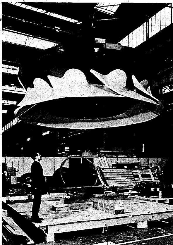
Fig 3.25 The same Deriaz runner shown in fig 3.24 but with the blades in the closed position. Photo by courtesy of GEC Turbine-generators Ltd
