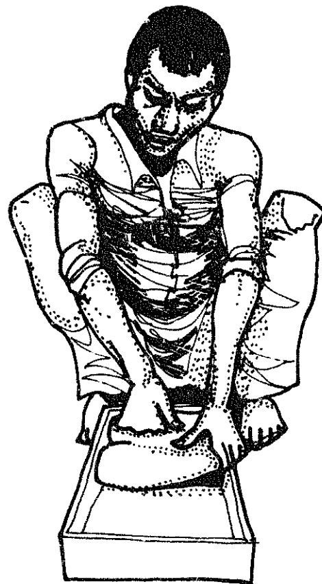
Stove fabricator makes connecting tunnel slabs in wooden former
