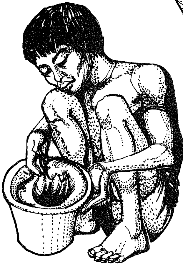
Figure 12.18. Moulding Thai stove liners.
