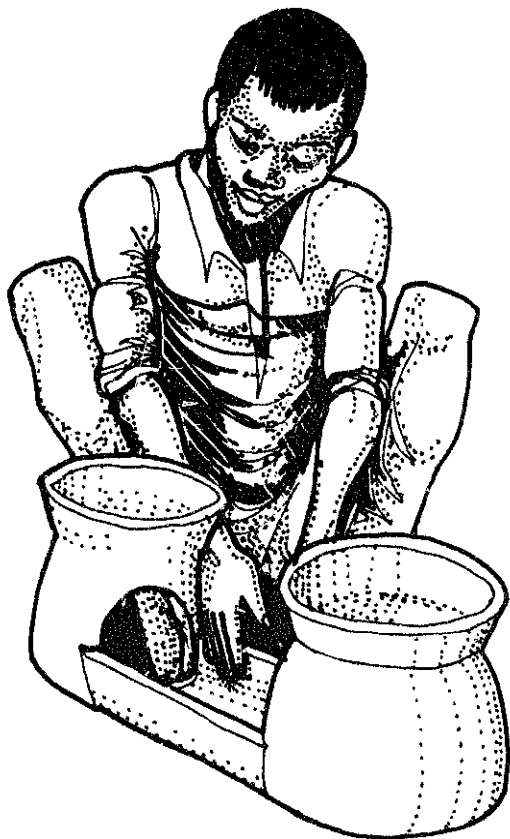
Tunnel floor connected and openings cut out
