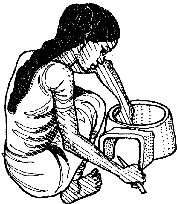
The firebox entrance is cut out
