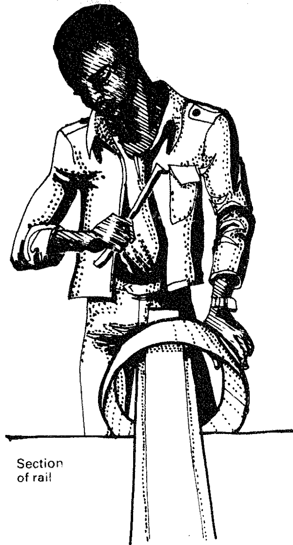
Figure 12.25. Finishing a rolled cone. Kenyan artisan using a flat bar made from a vehicle leaf-spring.
