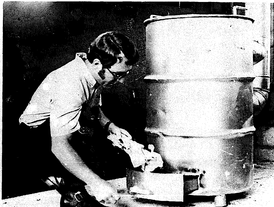
Lighted paper is inserted into the drawer to ignite the sawdust stove.
