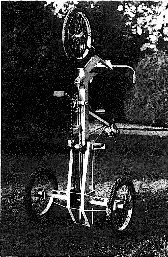
Figure 2-5 Up-ended view of Oxtrike chassis showing ability to park in a small space, easy inspection of transmission and brakes, and ability to tip out the load. Note Sturmey-Archer three-speed hub gear with double adjustment for primary and secondary chains.
