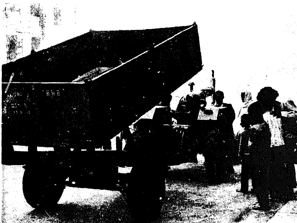
7. The simple tractor and trailer, used for secondary collection in Kathmandu, has hydraulic tipping gear. It was manufactured in India.
