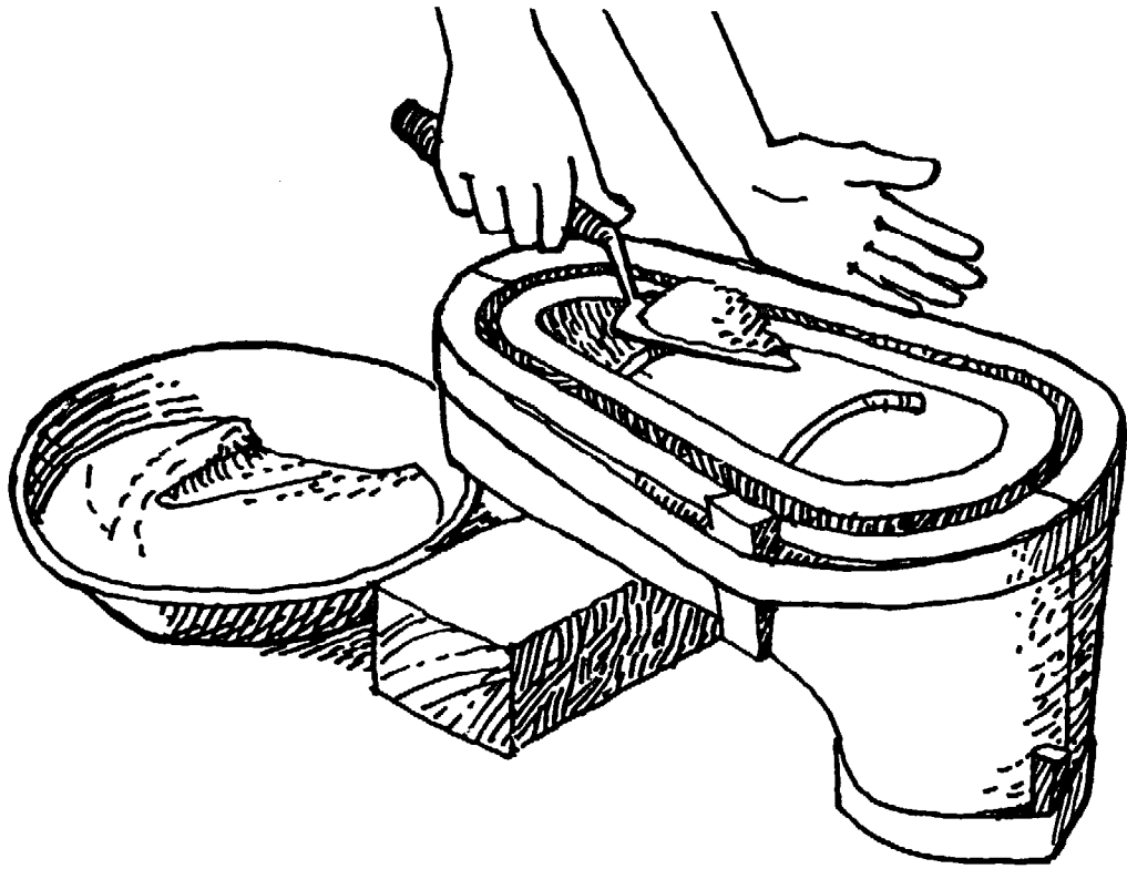
Figure 90 Casting the pan
