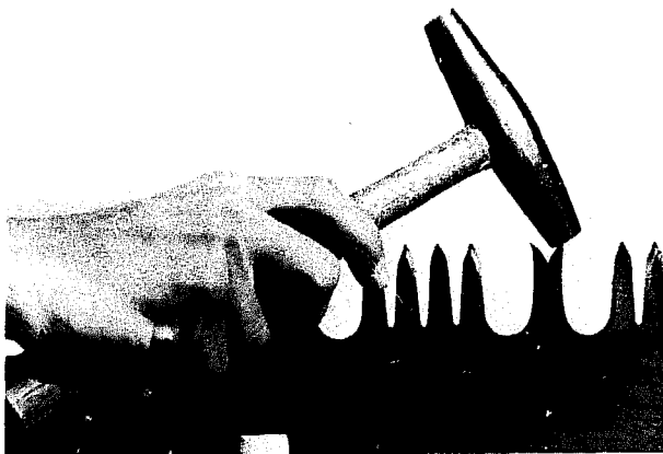
Striking the inside face of the raker tip with a hammer.
