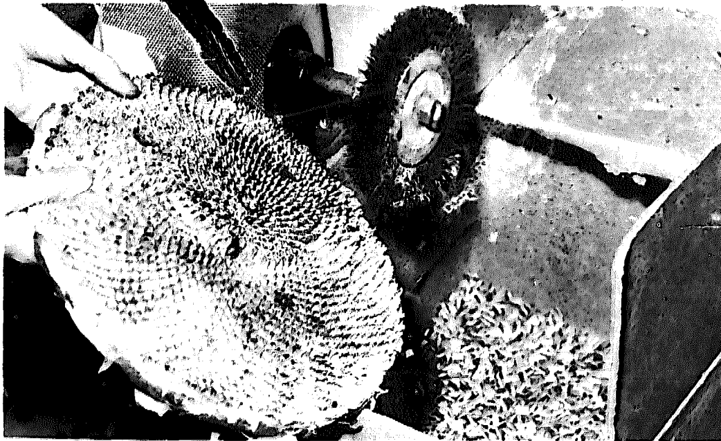
A home-improvised arrangement, such as this wire brush attached to a small electric motor, can simplify removing the seeds from the pods—often a difficult and tiring task for gardeners with a large quantity of sunflowers to harvest.
