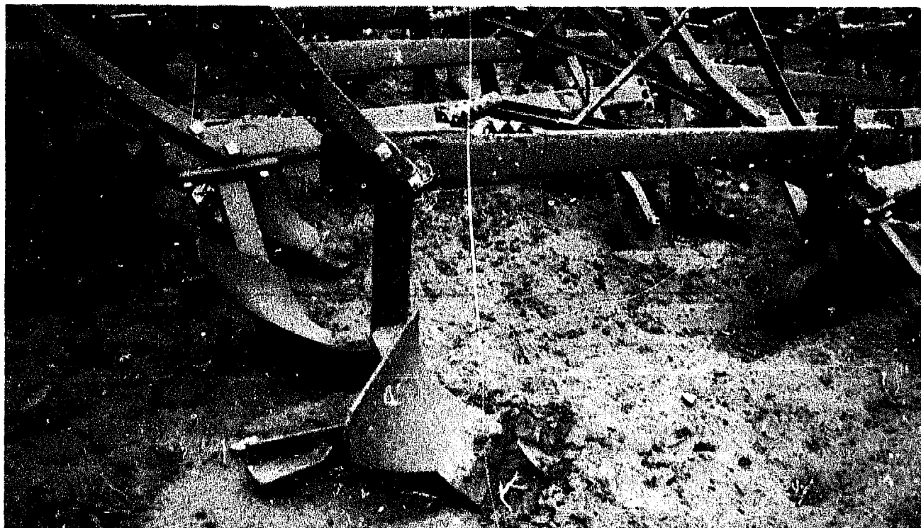
Fig. 11-6: Stockpile of plows imported into Mozambique by a donor-assisted project. The plows have numerous technical defects: for example the mouldboards and shares have no bolts but have been welded into place, making replacement in a small village almost impossible.
