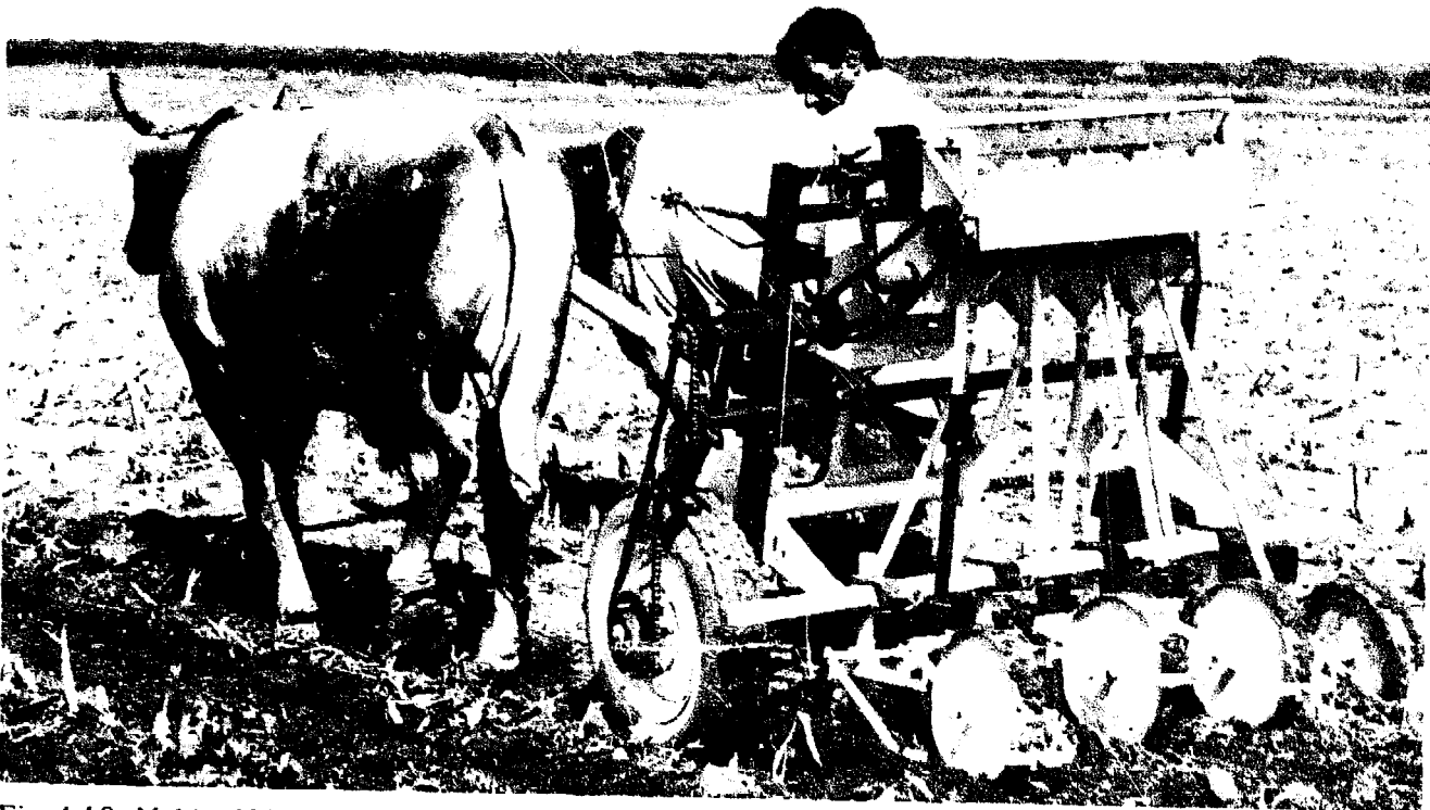
Fig. 4-10: Mekins Nikart with fertilizer-planter (Photo: ICRISAT archives).
