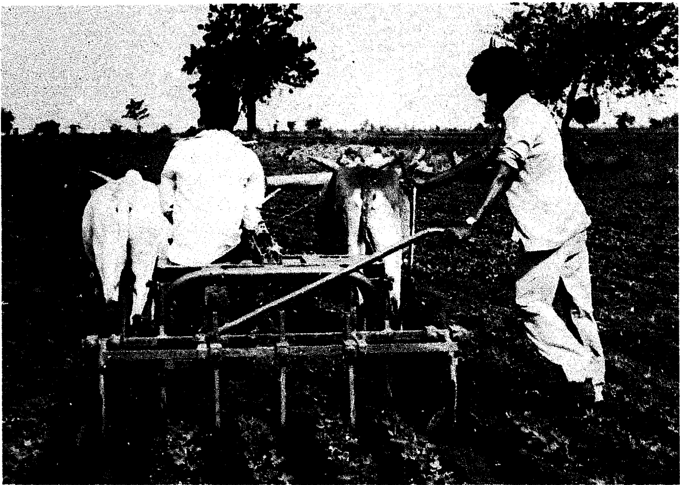
Fig. 4-14: Tropicultor with steerable weeder being used in on-farm verification trials in India. (Photo: ICRISAT archives).
