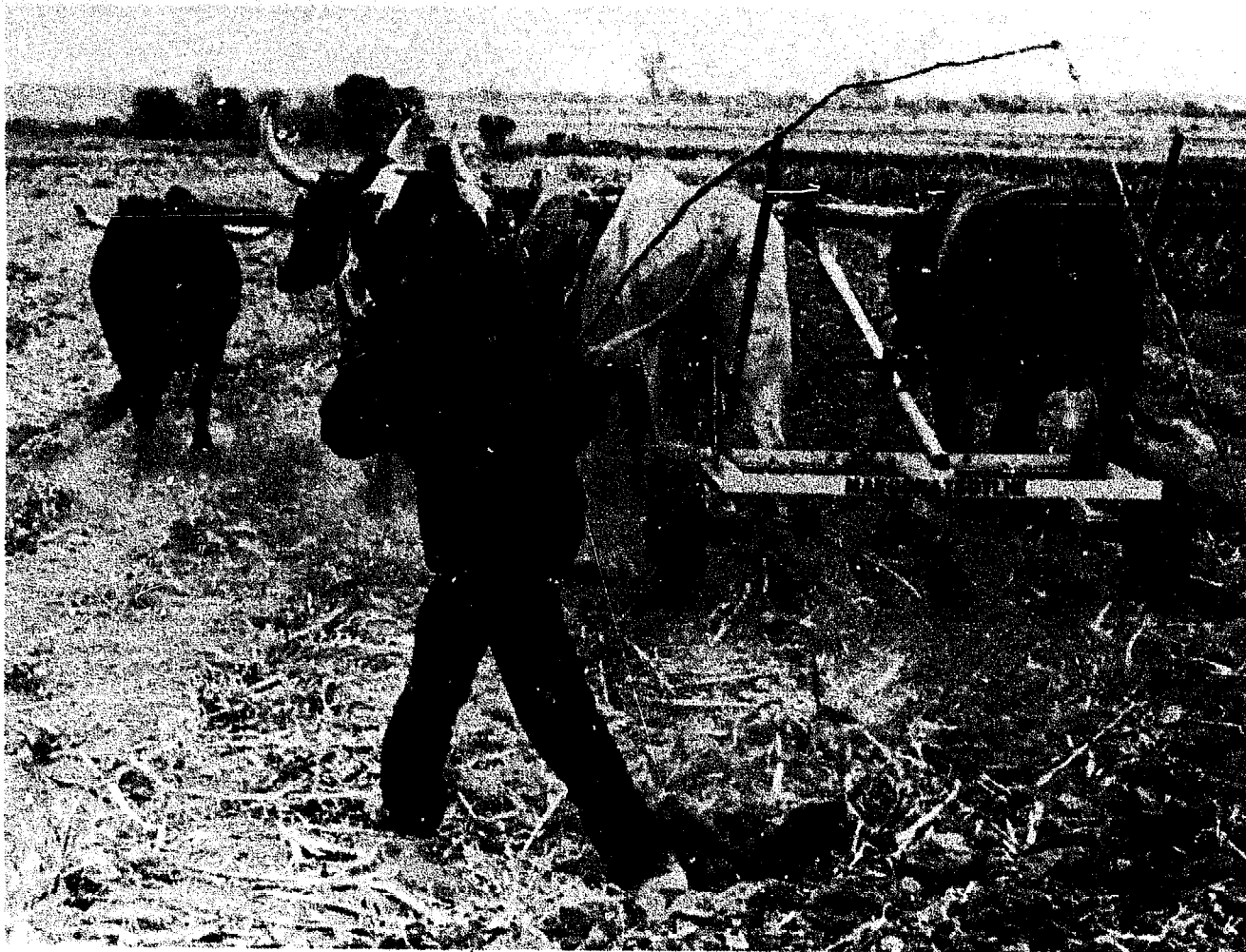
Fig. 3-17: Mochudi toolcarrier "Makgonatsotlhe" pulled by six oxen in an attempt at post-harvest sweeping during on-farm evaluation, Botswana, 1977. (Photo: FMDU archives).
