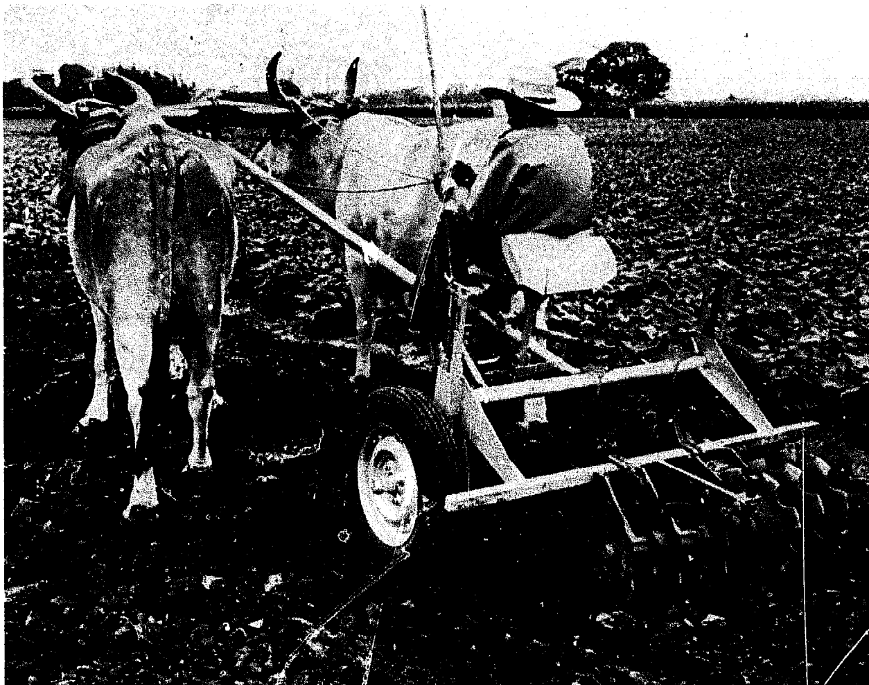
Fig. 6-7: Yunticultor with disc harrow in Mexico. (Photo: ICRISAT archives).
