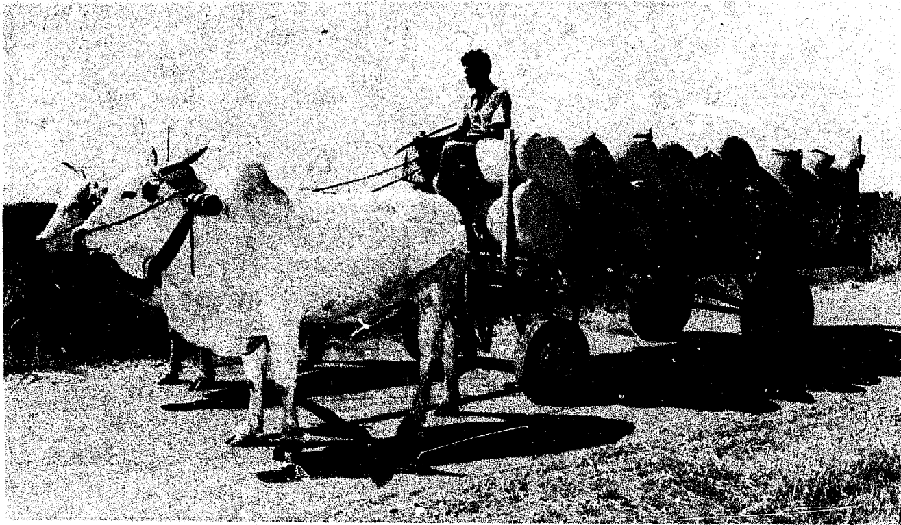
Fig. 4-5: Tropicultor fitted with four-wheel trailer, ICRISAT Centre. (Photo: ICRISAT archives).
