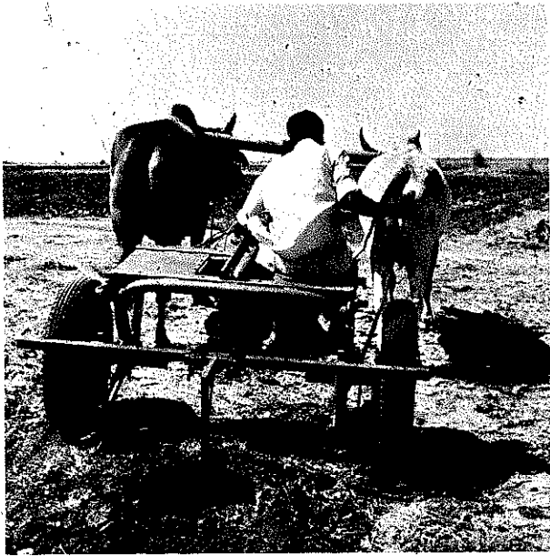
Go up to the end of the field and lift the toolbar.
