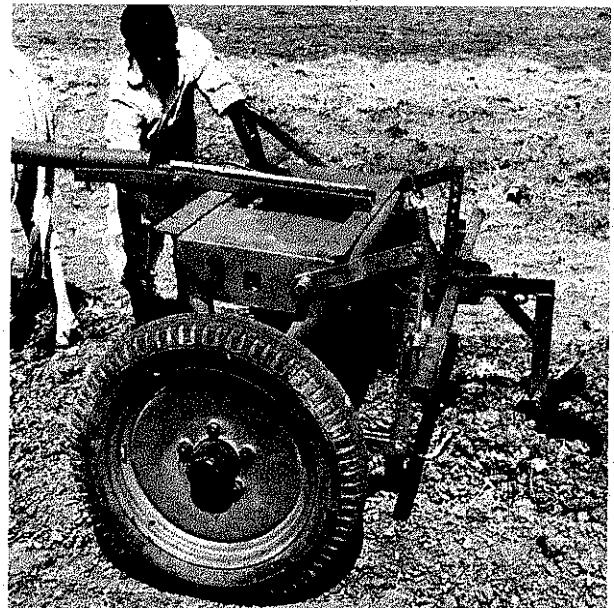
... make it vertical by turning the pitch adjustment screw.
