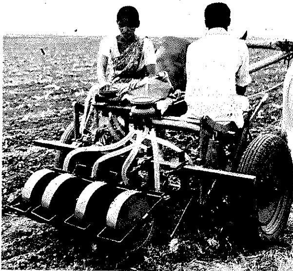
One person, in addition to the operator, is required to sit on the Tropicultor facing rearwards to drop the fertilizer by hand into the front bowl.
