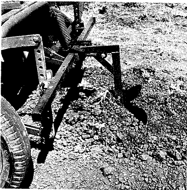
Start moving again and check if the ridger standard is vertical. If it is not, as shown here, ...
