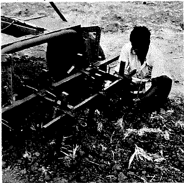
Measure the height of the projection and make it equal for all the tines.
