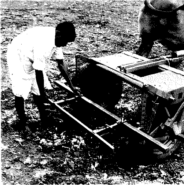
Fit the steerable toolbar to the main toolbar and insert the locking pins.
