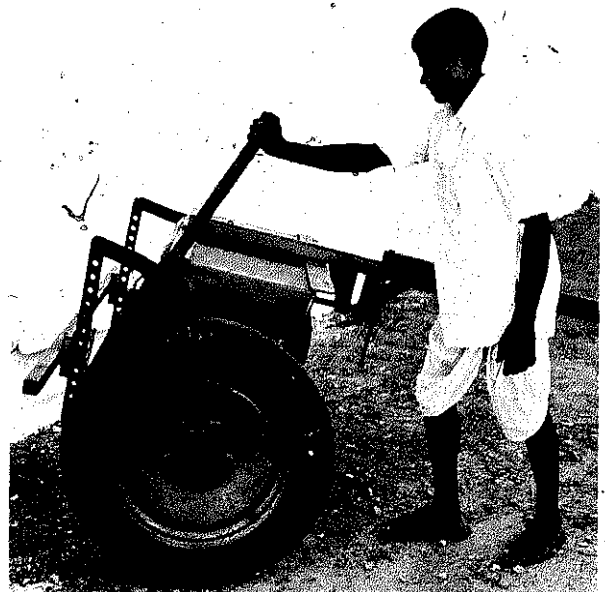
Check that the lifting handle functions properly in the extreme forward and rear positions: the toolbar should lock firmly in both positions,
