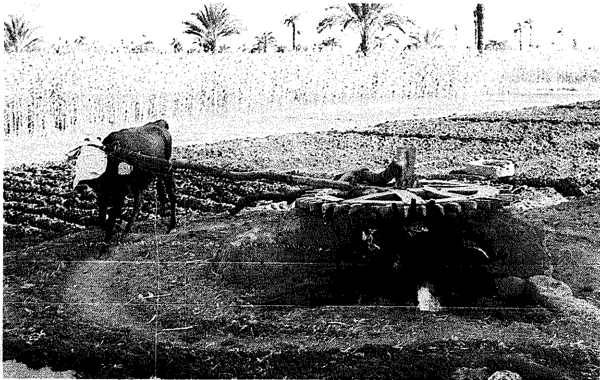
Fig. B/II/64: Wooden capstan with one pair of gears for conveying water. (Photo: GTZ Archives)
