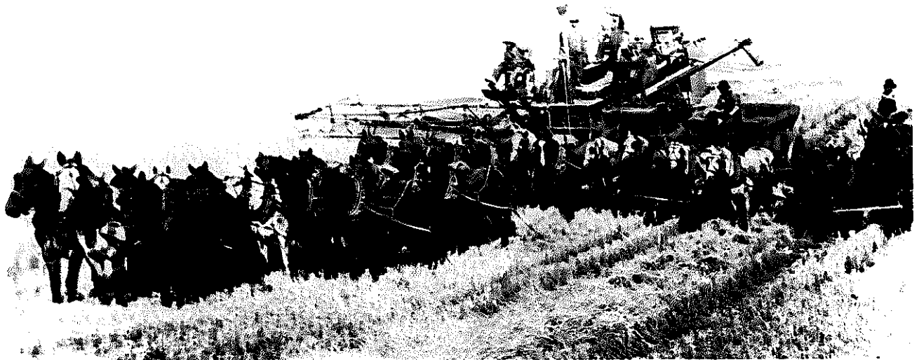
Combining with a twenty-five horse hitch near Walla Walla, Washington, 1917. (National Archives.)
