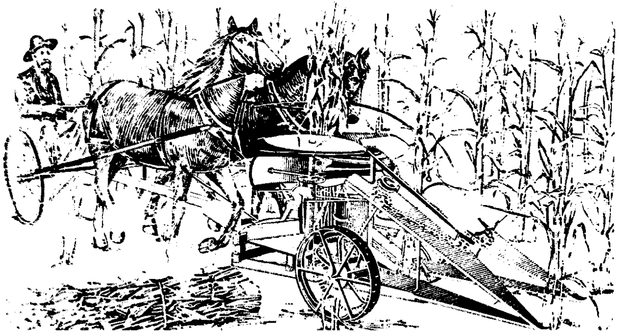
Above: The Peck corn binder operated in front of a two-horse hitch. It was the first satisfactory corn binder.
