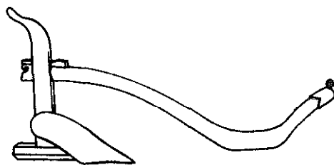
FIGURE 42. - Kedah plough (Malaysia) with improved share design.
