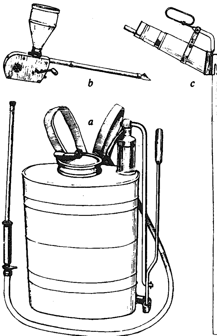
FIGURE 82. - Sprayers and dusters: (a) knapsack sprayer; (b) fan-type duster; (c) bellow-type duster, also used for pollination of date palms.
