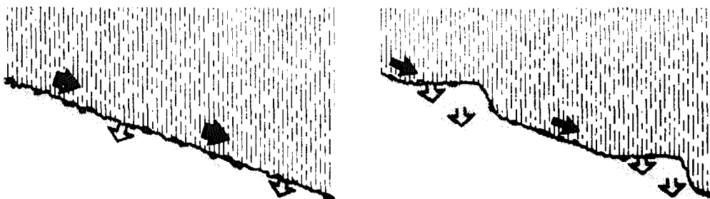
Fig.8 Run-off interception with ridges
