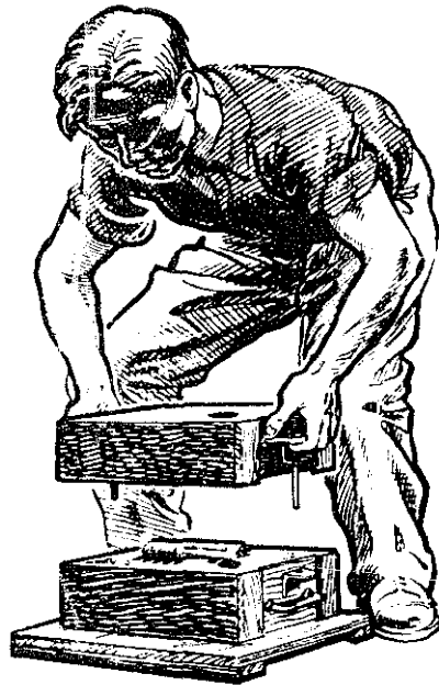
Fig. 21. Closing a large mould.
