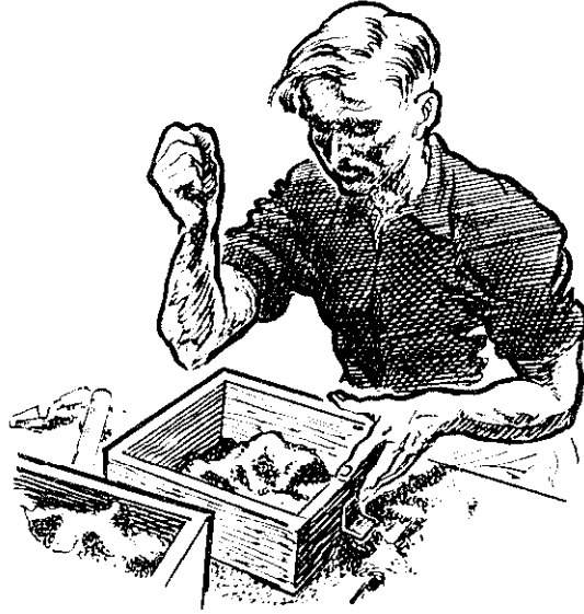
Fig. 57. Moulding by sand slinging.
