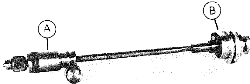
Fig. 10. The drilling spindle in use on the saddle of the Myford lathe
