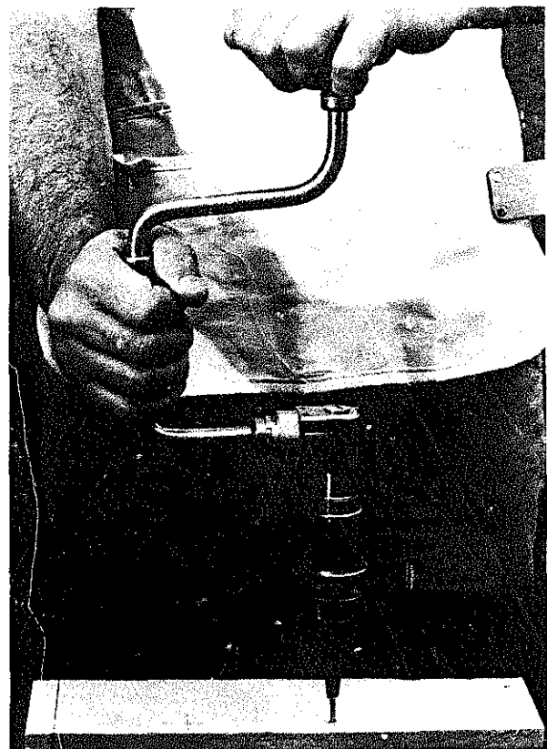
Fig. 12-20 Driving a screw with a screwdriver bit.
