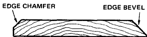
Fig. 8-38 Comparing a chamfer to a bevel.
