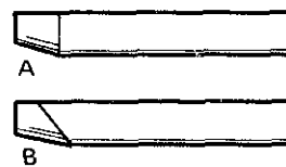
Fig. 9-44 (A) Correctly ground bevel, (B) incorrectly ground bevel.
