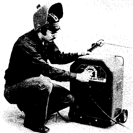
Fig. 4-5. A typical small AC transformer welder for light-duty and limited-service welding.
