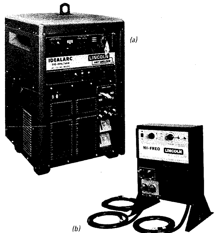
Fig. 4-29. A transformer-rectifier welder (a) designed for AC-DC TIG welding or for AC-DC welding with consumable covered electrodes; (b) a high-frequency generator for adapting an AC or DC metal-arc welder for use with the TIG process.
