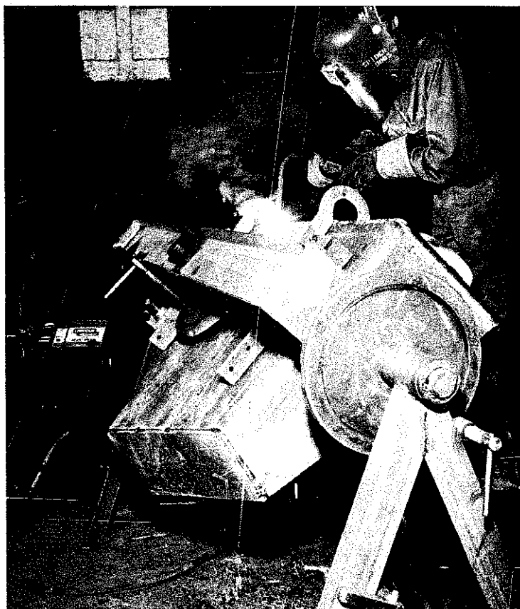
Fig. 4-47. C clamps attached to the work provide a good ground and help maintain the uniform voltage and current control needed for semiautomatic welding.
