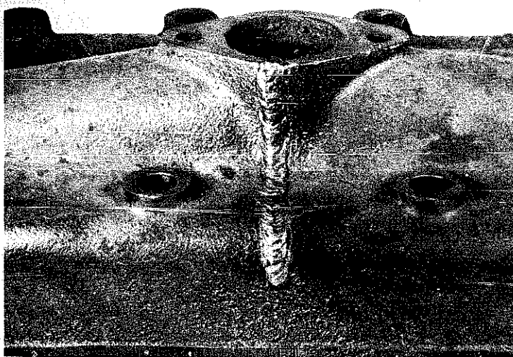
Fig. 8-1. Repair of a crack in a cast-iron cylinder head with an ESt electrode.
