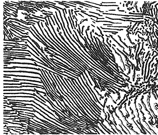
Fig. 8-25. 0.85 percent carbon steel, all pearlite. Magnified 2800 times.
