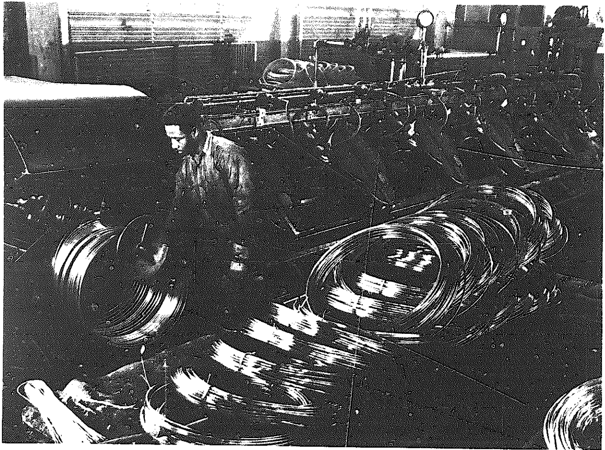
Fig. 16-7. Small diameter soft copper bar being drawn on a special machine. (Chase Brass and Copper Co.)
