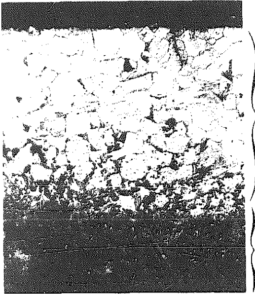
Fig. 9-20. Decarburized tool steel, magnified 200 times. Surface of steel is white against black; The decarburized zone is the middle-section; and the high-carbon zone is at bottom, dark.
