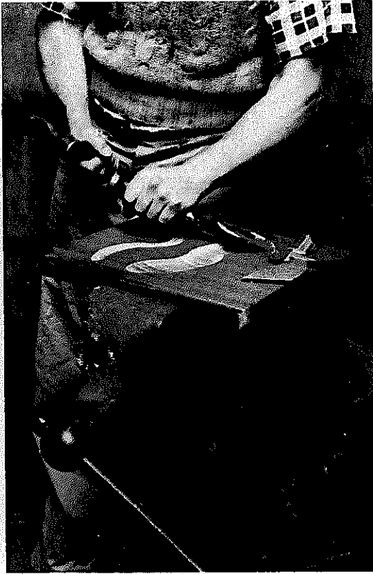
Testing cone design of gouge, cutting an S-curve through splintery, soft, redwood board. The bevel edge is on the outside. The slant of the edge is an original design feature described in Chapter 12.
