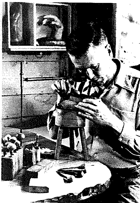
The engraving reproduced here was engraved on endgrain wood, using traditional burins. The burin's flat upright allows it to slide along the thumb during the tool's cutting strokes.
