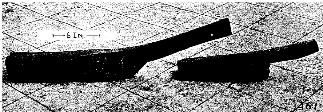
FIG. 433. WOODEN BATS USED IN BEATING DOWN (SOLIDIFYING) CHINESE COMPOSITION PAVEMENTS. The smaller one is 19 inches long and the surface resting on the ground 12\frac{1}{2} inches long and 4\frac{1}{2} inches wide. The larger one is 2 feet 8 inches. Photographed in Kien'Chang, Kiangsi.
