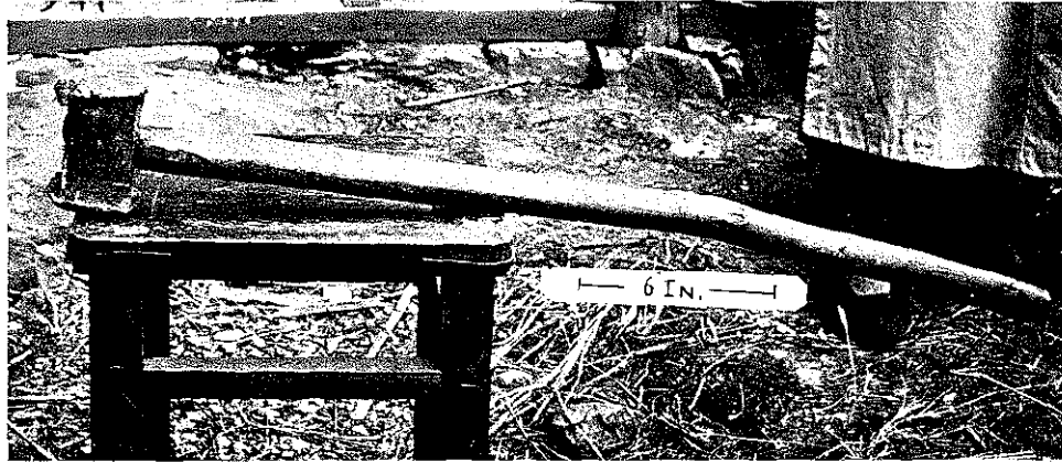
FIG. 13. COAL MINER'S LONG HANDED GAD HAMMER. One miner holds the point of the handled iron gad, Fig. 12, against the solid coal seam, while another miner strikes the flat gad-face with this hammer.
