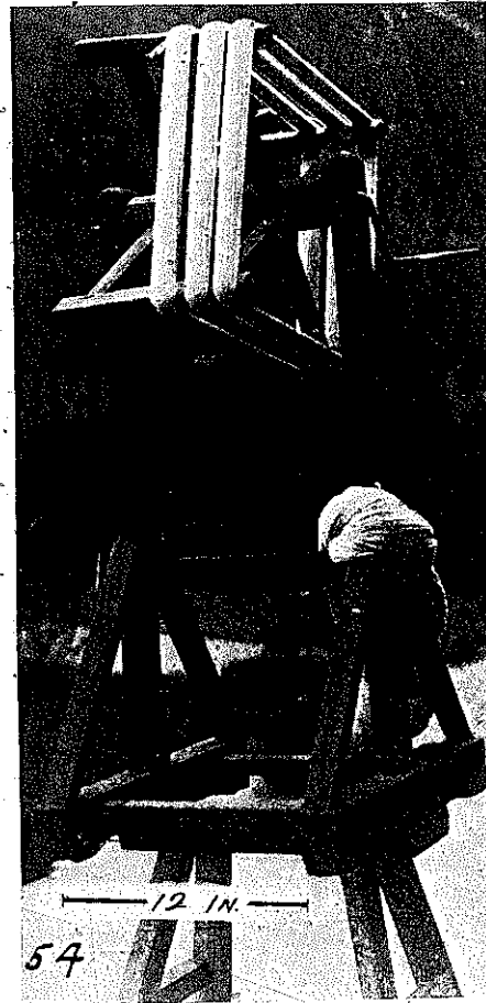
FIG. 262. HANK REEL FOR WINDING UP FRESHLY TWISTED COTTON THREAD.
