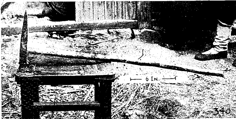
FIG. 12. COAL MINER'S HANDLED WEDGE, OR GAD. Where space permits, one man holding the instrument by its handle, sets its sharp point upon the solid coal, while another drives the iron point into the seam to split it by striking the flat face of this tool with the iron hammer shown in Fig. 13.
