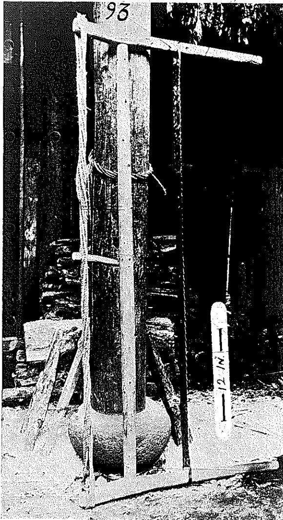
FIG. 322. BOARD SAW OR PIT SAW.
