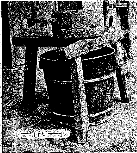
FIG. 160. QUERN FOR WET GRINDING USED IN MAKING BEAN CURD.
