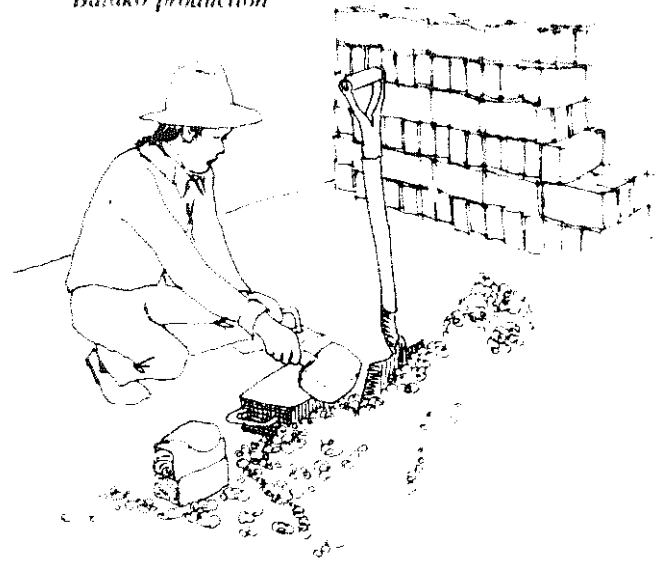
The trass and lime mixture is pounded into the mold with a broad wooden mallet.
