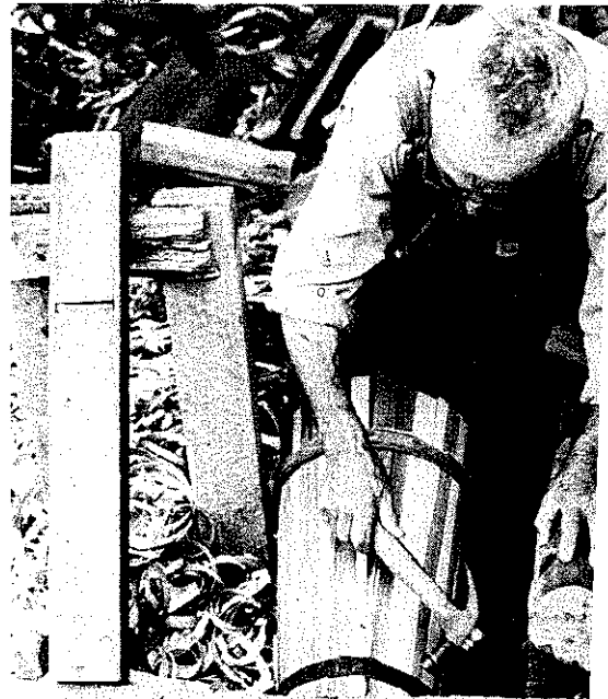
PLATE 347 Step 5: Use a hammer to fit in the last stave. If it won't fit, adjust the other staves with the jointer. A tight fit is absolutely necessary.
