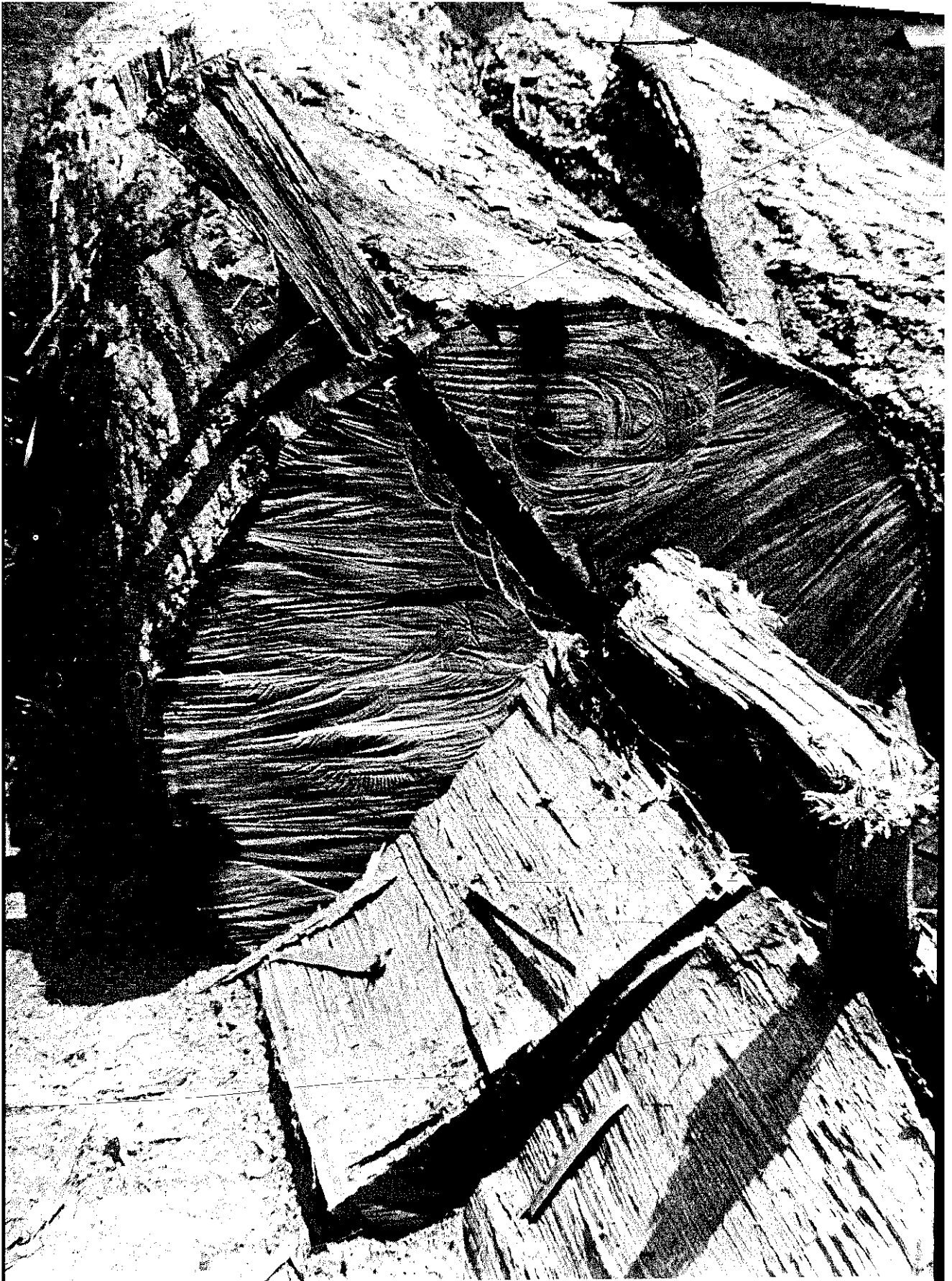
PLATE 19 The two wooden wedges already driven into this huge trunk have begun to split it in half.
