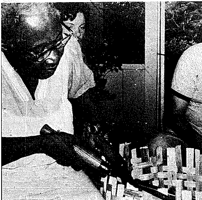
PLATE 165 At the top, the ends of the ribs will probably be uneven. Before the rim can be made, these must be trimmed off straight. This can be done with a knife or, as shown here, with a pair of hedge clippers.
