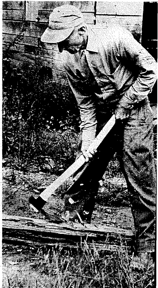
PLATE 17 The proper stance to use when working with a foot adze is demonstrated by Bill Lamb. The handle of the adze has a double curve for ease in working.
