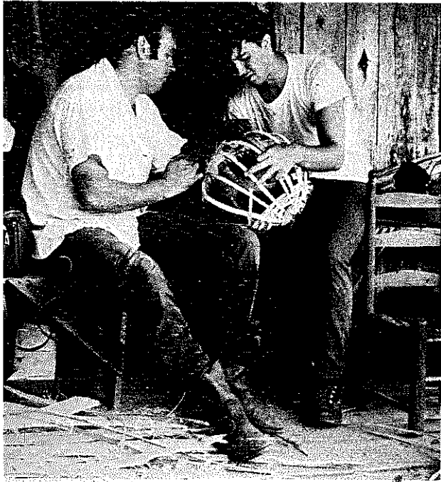
PLATE 177 . . . inserting ribs until there are five on either side of and parallel to the main hoop.
