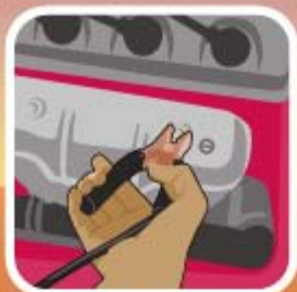
Ground to the engine block.
