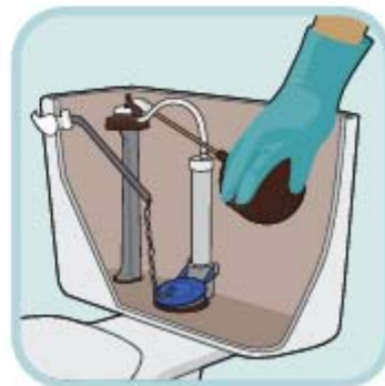
Check the flush ball for leaks.
