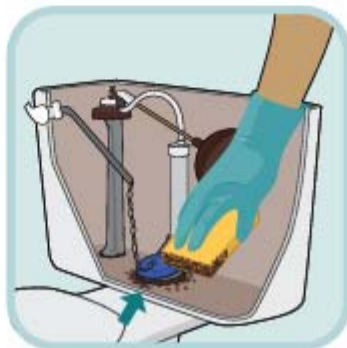
Clean the flush valve seat.
