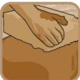
Place bricks on the mortar.
