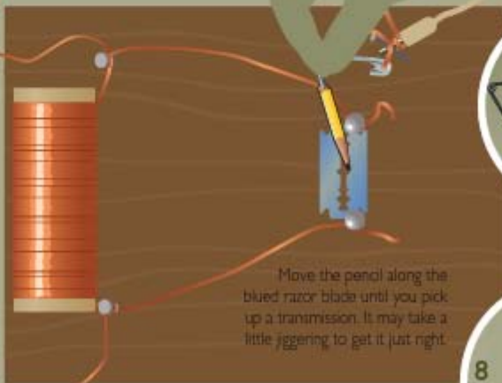
Expose the wire's other end—it acts as an antenna.
