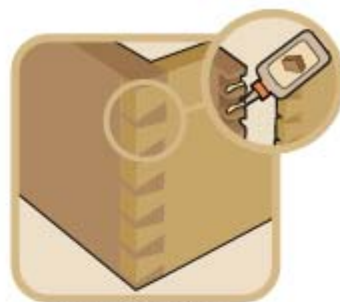
Cut the tail board joint.
