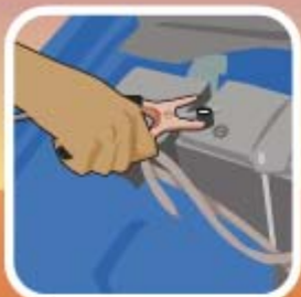
Link to the booster battery.
