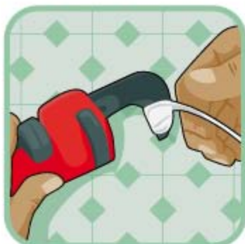
Cover the wrench with pipe tape.
