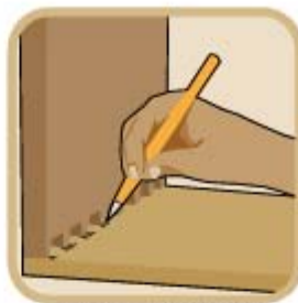
Transfer to the tail board.
