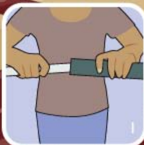
1 Sheath the pipe with foam.
