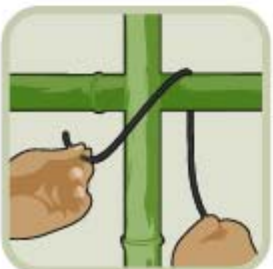
Weave around the joint.
