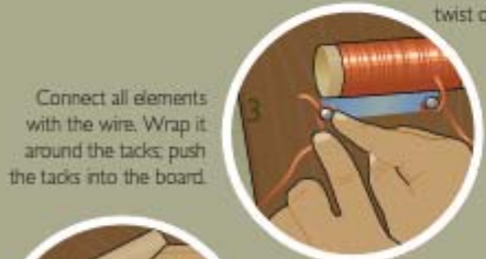
Thread the wire through a hole in the tube, then wrap it around the tube.
