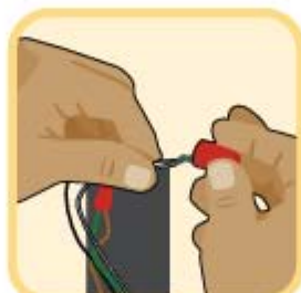
Insert the wires into wire nuts.
