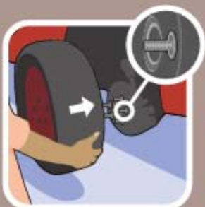
Put a spare over the studs.
