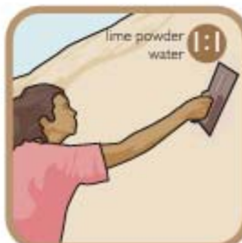
Seal with a lime wash.
