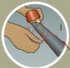
Thread the wire through a hole in the tube, then wrap it around the tube.
