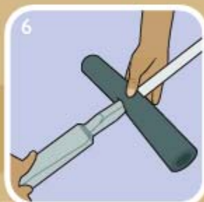
6 Slide onto the bare pipe end.
