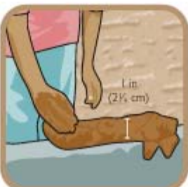
Spread the mortar.
