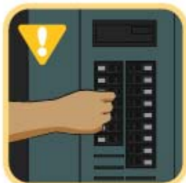
Turn off the power to the light.
