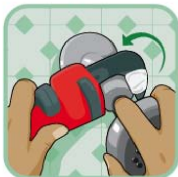
Loosen the showerhead from the pipe.
