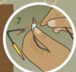
Wrap the wire around the safety pin and the earphone's receptor.
