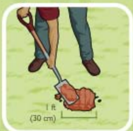
Dig holes for the fence posts.
