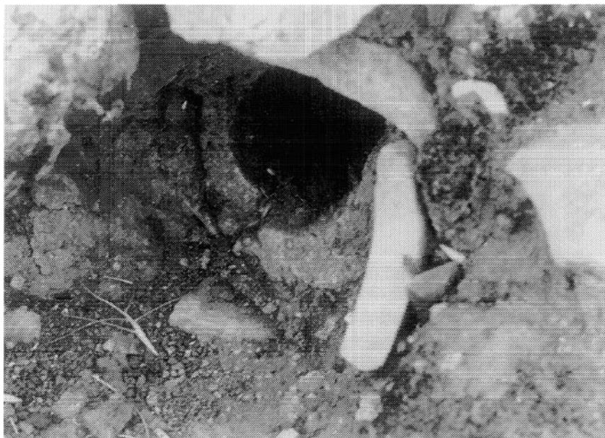
**Figure 16.4.** Broken pipe mended by being wrapped in additional terra-cotta pieces. This was the supply pipe for the street fountain in the northwest corner of the Agora, Morgantina. The inside pipe was approximately 10 centimeters in inner diameter.
