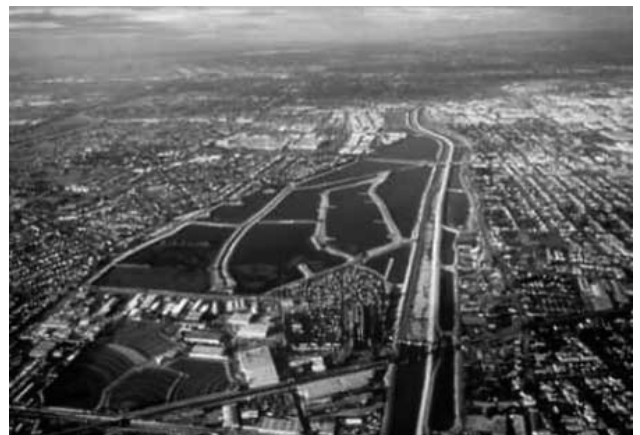
For over 35 years, in the Montebello Forebay Groundwater Recharge Project, recycled water has been applied to the Rio Hondo spreading grounds to recharge a potable groundwater aquifer in south-central Los Angeles County.
