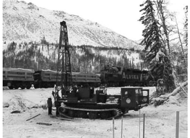
Figure 1. Rotary drilling rig used to assess shallow spillage from train derailment area at mile 262 (Photo P045; EPA).
