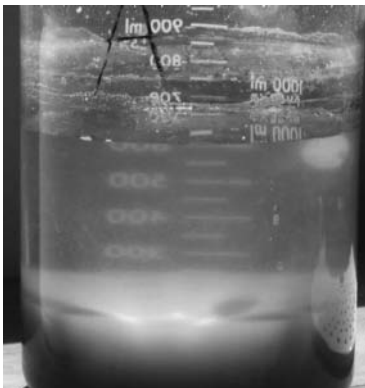
Figure 4. Precipitation of solid insoluble chromium into a sludge blanket.
