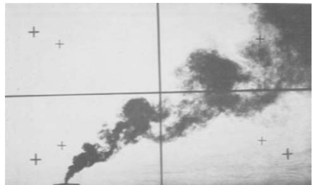
Figure 4. A single port buoyant jet in cross flow deflected by the ambient current (near-field flow).
