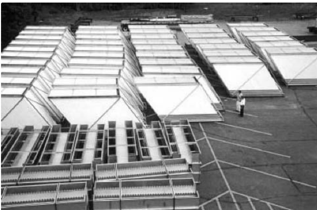
Figure 3. Plate settlers for installation (Source: U.S. Filter).
