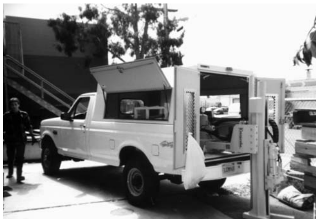
Figure 3. Direct push technology rig (Courtesy FAST-TEK).
