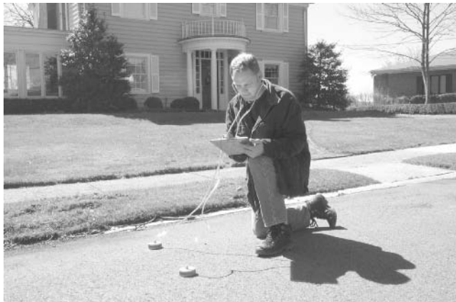
Figure 1. Shawn Menear, a graduate student in technology education at west virginia university, uses geophones to listen for water main leaks. Similar to a doctor or nurse's stethoscope, geophones are an inexpensive leak detection device used by water utilities.
