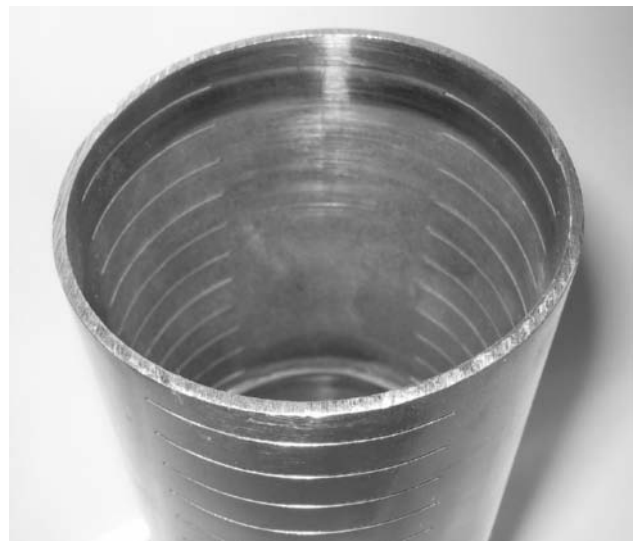
Figure 4. Horizontal machine-slotted screen.
