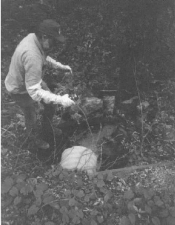
Figure 3. Fluorescein dye introduced into a sinking stream that flows across recharge units of the Capon Warm Springs Complex in Hampshire County, West Virginia.
