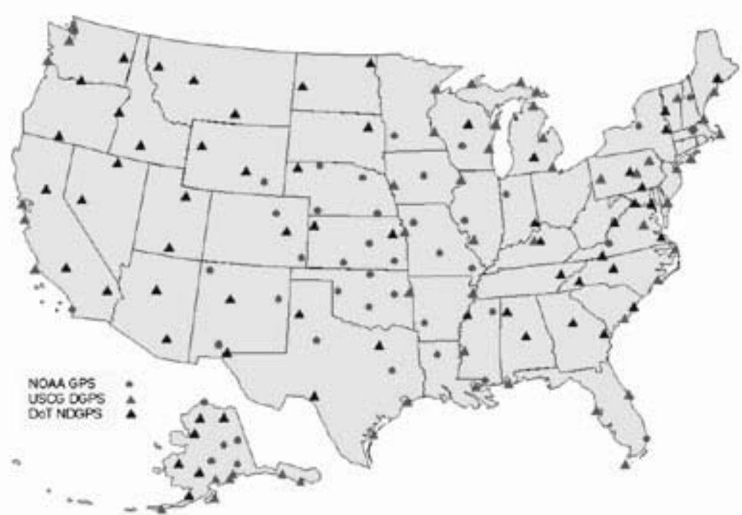
Figure 12. Expected configuration of the NOAA/FSL GPS-IPW Demonstration Network by 2005. Sites in Hawaii and the Caribbean Sea are not shown.
