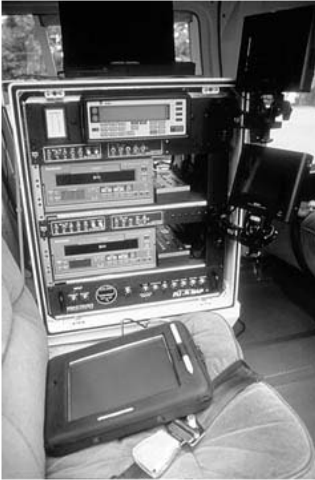
A laser scanning rangefinder make a hefty instrument package for a helicopter (Photo courtesy of New Orleans District)
