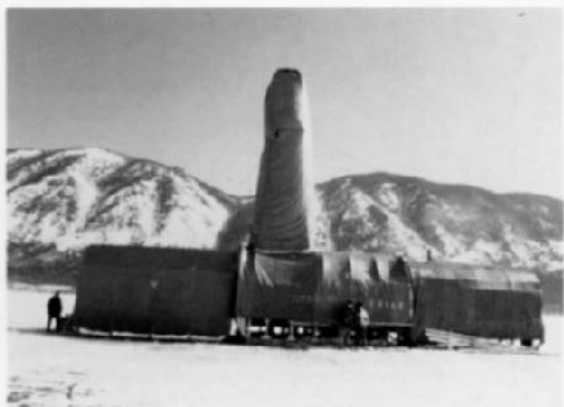
Ice-based drilling rig being tested on a small marginal lake in North Baikal. Photo by D. Williams.
