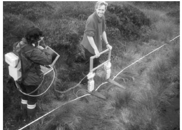
Figure 2. Ground penetrating radar being used in the field to detect soil pipes. Photo by Vincent Holden.
