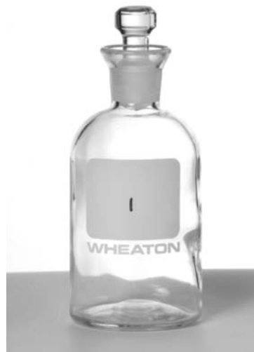
Figure 1. Standard 300 mL BOD bottle.
