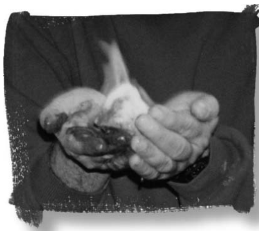
Figure 4. Burning the methane that is released as a gas hydrate sample decomposes. Hands belong to Robert Collier (College of Oceanic and Atmospheric Science, Oregon State University). Picture taken by one of the authors (M. Torres).
