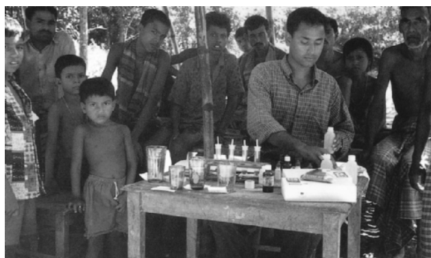
Figure 3. Testing for arsenic in drinking water using test kits at a village.
