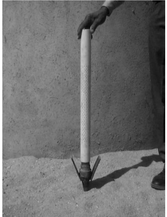
Figure 6. Well points suitable for small-scale sand-abstraction system.
