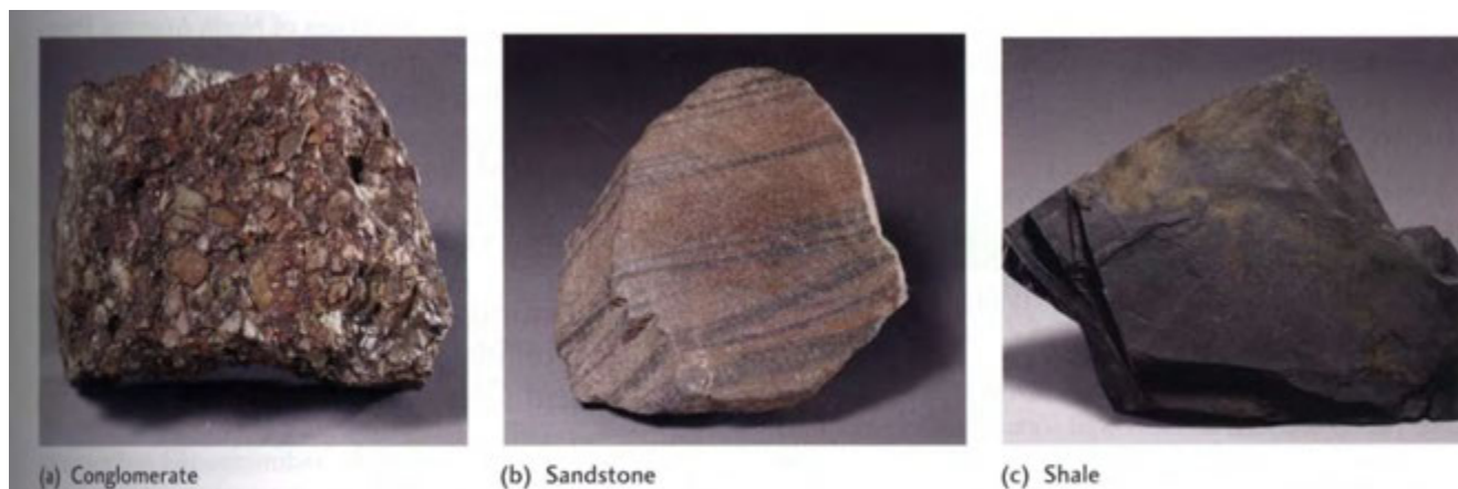
Figure 5.15 Clastic sedimentary rocks. [Conglomerate and sandstone: John Grotzinger/Ramón Rivera-Morez/MIT. Shale: John Grotzinger/Ramón Rivera-Morez/Harvard Mineralogical Museum.]
