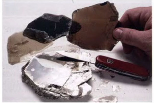
bonding the two tetrahedral layers into a sandwich. Cleavage takes place between composite tetrahedral–aluminum hydroxide sandwiches. The photograph shows thin sheets separating along the cleavage planes. [Chip Clark.]
