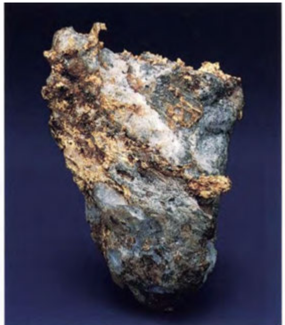
Figure 3.27 Gold occurring in the free state (native gold) on a quartz crystal. [Chip Clark.]
