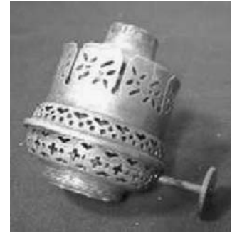
BURNER FOR ARGAND LAMP The novel burner design by Aimé Argand (not the Argand who developed representation of complex numbers) holds a circular wick whose flame receives oxygen from both inside and out, burning more brightly than a simple linear wick.
