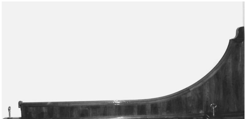
MODEL OF A CYCLOID This wooden model shows a track shaped in the famous curve known as a cycloid. One of several alternate names for the cycloid, the isochrone ("same time") is illustrated by the model — an object placed anywhere on the track will slide to the bottom in the same amount of time as an object placed at a different point on the track. This property was exploited by Christiaan Huygens — who discovered it — to create a pendulum that, because its weight is constrained to fall in a cycloidal path instead of an arc of a circle, will have exactly the same period for any amplitude.
