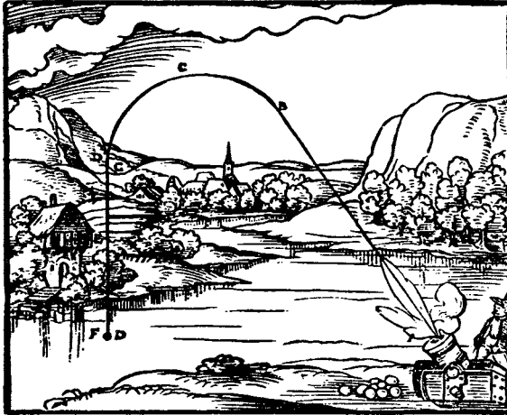
Figure 10.1. An Aristotelian representation of a cannonball's trajectory. It illustrates the Aristotelian concept that the trajectory consists essentially of two separate motions, unnatural (away from the ground) and natural (toward the ground). In this figure the transition between unnatural and natural motions is a circular arc. (From G. Rivius, Architectur, Mathematicischen, Kunst , 1547).
