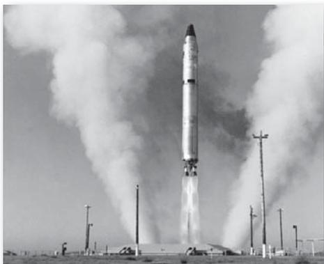
*Titan II rocket, lifting off from an underground silo. Developed as an intercontinental ballistic missile, the Titan II also served as a launch vehicle for the Gemini manned spacecraft missions and military and civilian satellites. U.S. Air Force; photograph provided by Donald Boelling*
