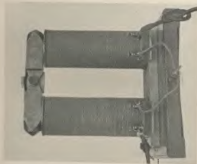
FIG. 12. Electro-magnet. The capsule of radium is fixed on the near side of the pole-pieces so that the rays pass between the poles to the screen on the far side.
