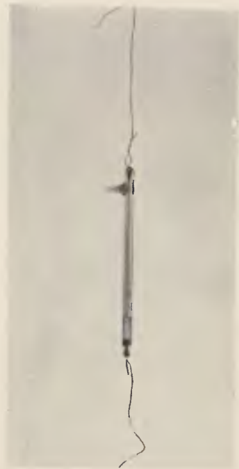
FIG. 21. Original Spectrum-Tube in which the formation of Helium from Radium was first observed.
