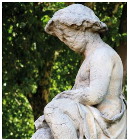
Effect of acid rain on stone The face of this statue has been obliterated by acid rain because the detail of the features had a large surface area, encouraging a reaction between acid and limestone.
