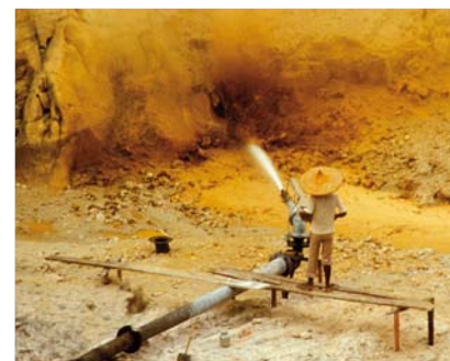
Mining tin ore with a high-pressure water jet Breaking up tin ore with high-pressure jets of water—a process known as gravel pumping—is the most common method of mining tin in Southeast Asia. The method is highly economic for small, scattered deposits of ore.
