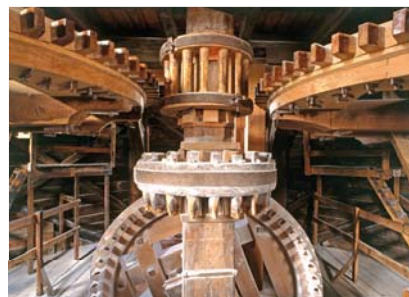
Bevel gears These change the axis of rotation.
