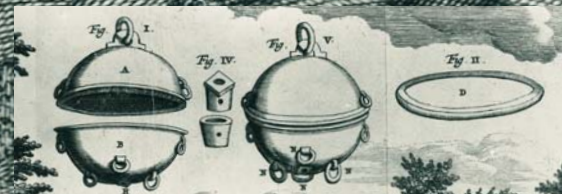
Creating the unbreakable seal Otto von Guericke pumped the air out of two copper hemispheres of around 20 in (50 cm) diameter sealed with a greased leather ring. Because this created a vacuum, there was no air pushing outward from the insides of the sphere, but there was pressure (atmospheric) pushing on them from outside, which forced the spheres tightly together.
